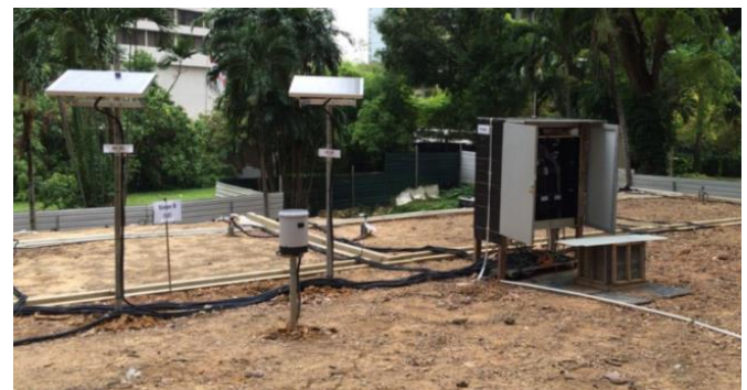
Figure 2 Data acquisition system used at the study site
