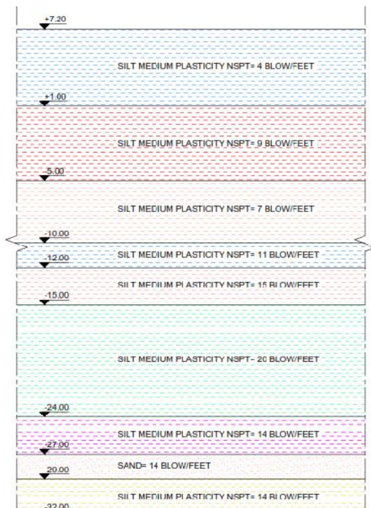
Figure 17. Soil Stratification of UP Bojong
