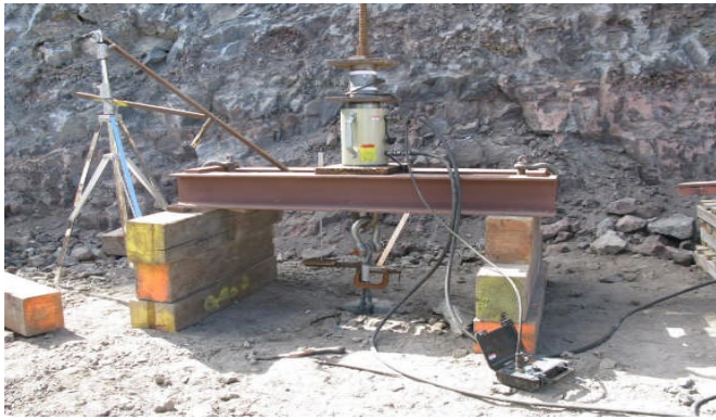
Figure 12. Example of a pull-out test to verify the designed length of the top anchors.
