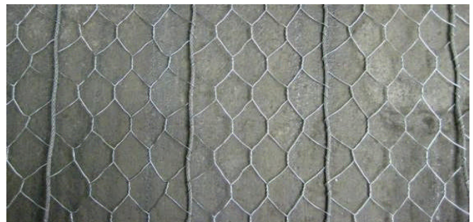
Figure 15. Detail of the cable woven in the double twist mesh to form the SteelGrid (the 8mm cables are interwoven in the mesh with 30 cm spacing in order to reach very high tensile resistance, up to 177 kN/m).
