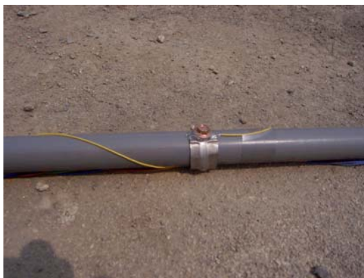
Figure 20 In-hole resistivity sensors for 3D RIP tests
