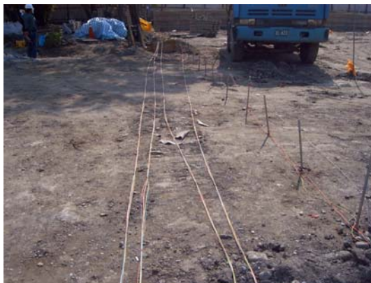
Figure 19 Probing posts for 2D RIP tests at ground surface
