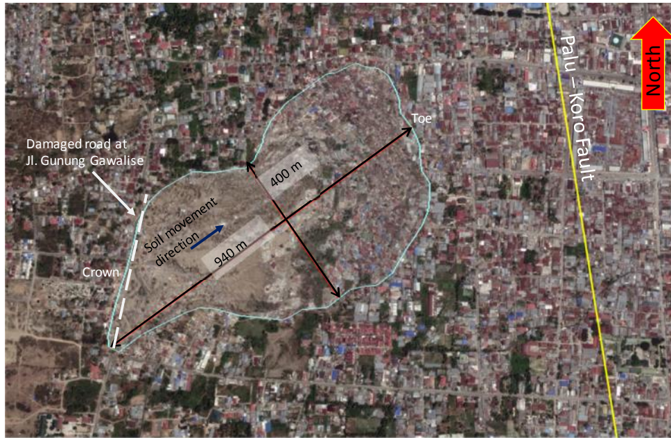
Figure 13 Estimated soil failure affected area in Balaroa
