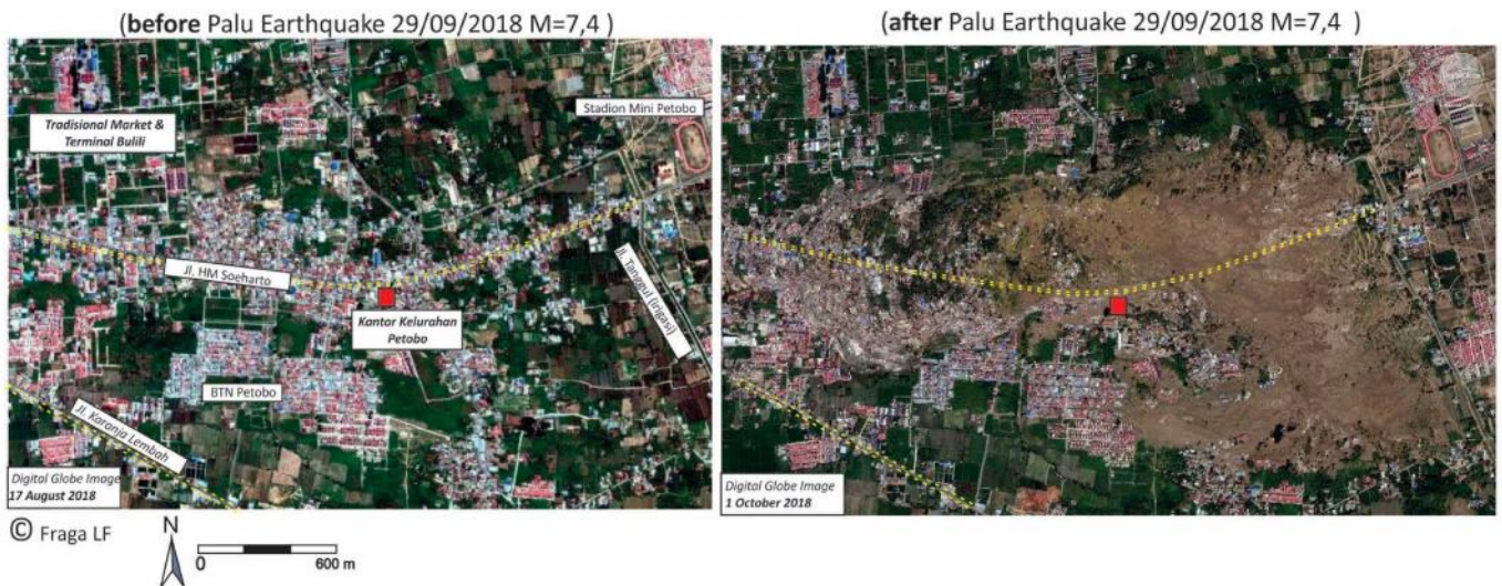
Figure 11 Liquefaction induced lateral spreading in Petobo village (Digital Globe)
