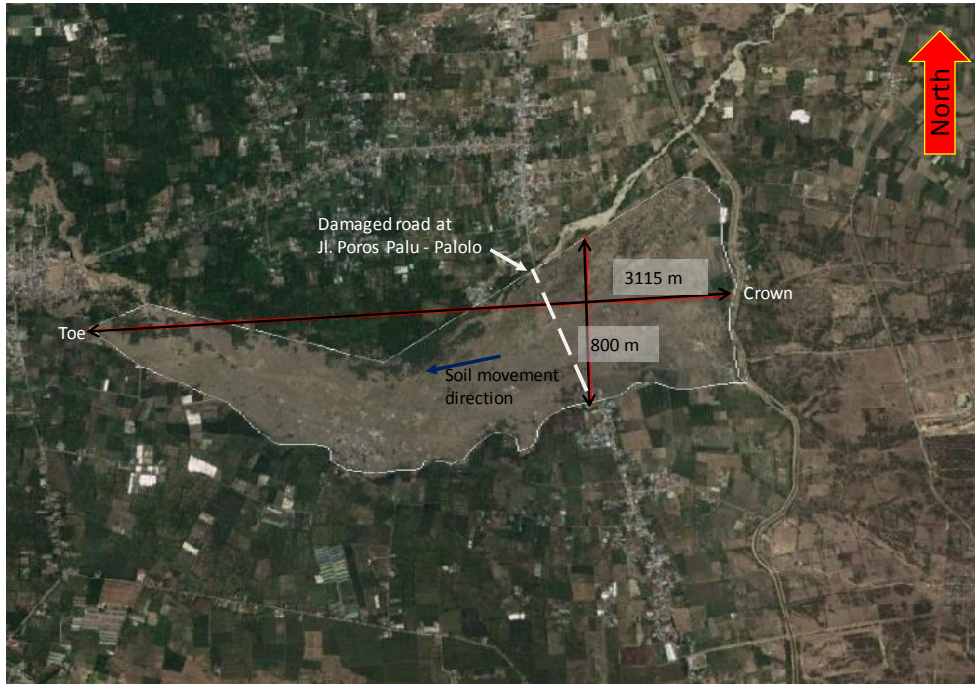
Figure 16 Estimated soil failure affected area in Jono Oge
