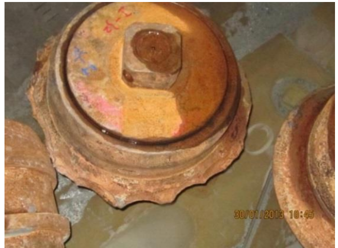
Figure 5 Damaged and abraded disc cutter, EPB TBM working in weathered Singapore granite
