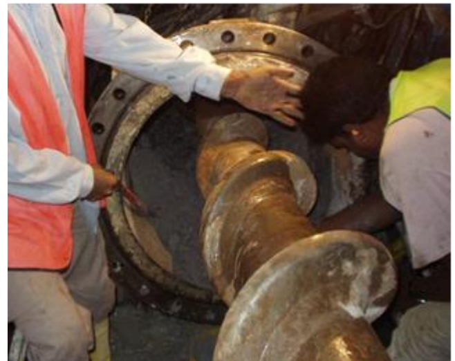
Figure 6 Badly abraded screw conveyor, DTSS, section in weathered granite
