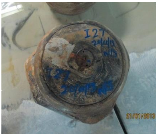
Figure 4 Damaged and abraded disc cutter, EPB TBM working in weathered Singapore granite
