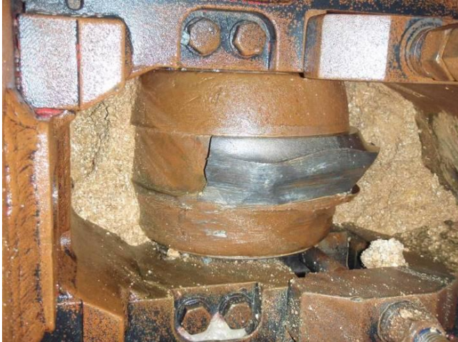
Figure 8 Damaged and abraded disc cutter, slurry TBM working in weathered Singapore granite
