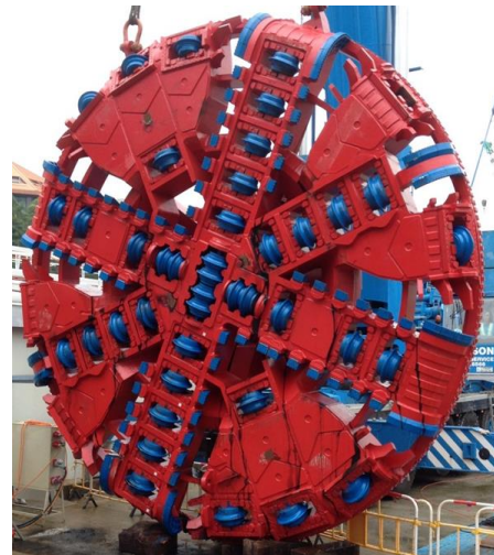
Figure 3 Typical mixed ground cutterhead used for a slurry TBM in Hong Kong
