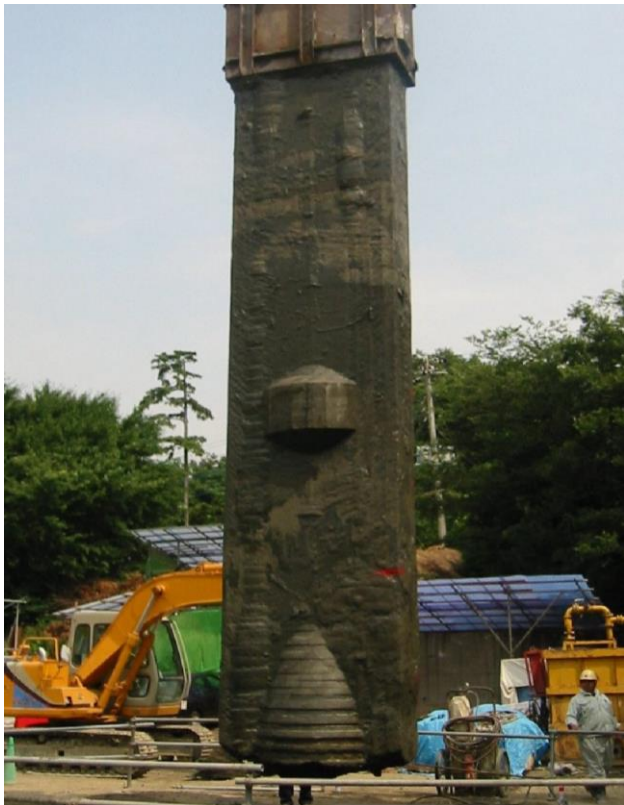
Photo 1 Test nodular diaphragm wall having nodular parts and pile base enlargements
