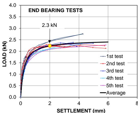
Figure 18 Load-movement curves of end bearing tests
