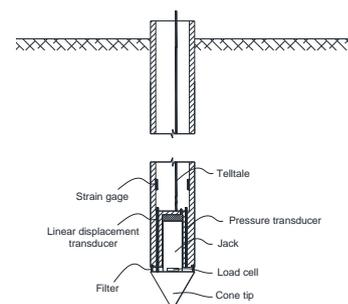
Figure 2 Scheme of novel CPT equipment
