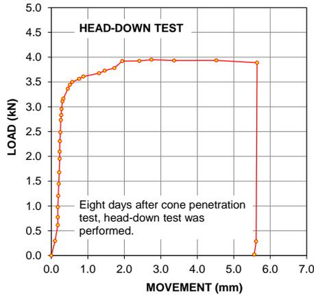
Figure 14 Load-movement curves of head-down loading test
