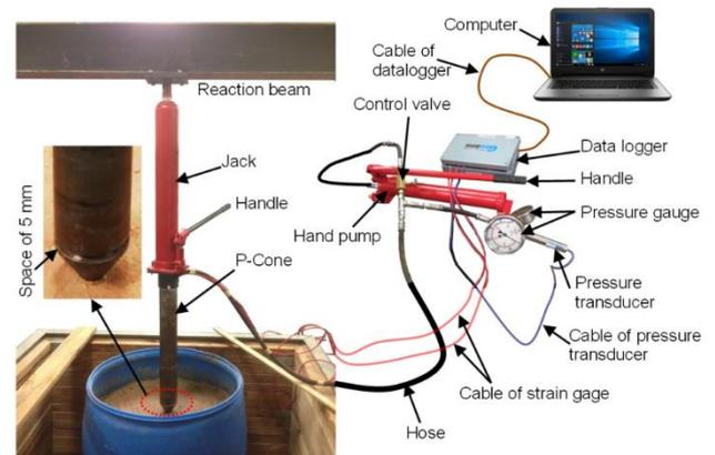
Figure 5 The operating principle and the measurement system of the P-Cone
