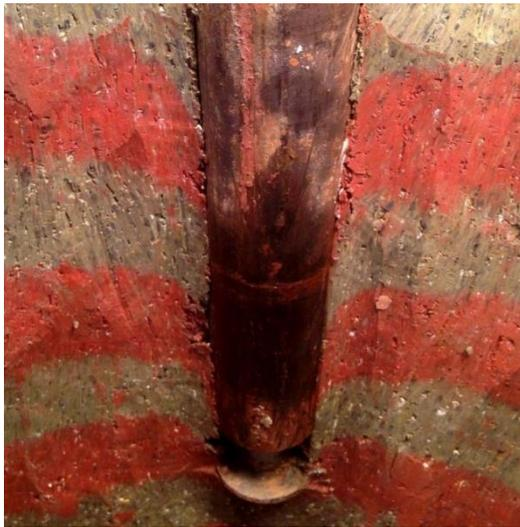
Figure 17 The failure surface of soil along the cone shaft
