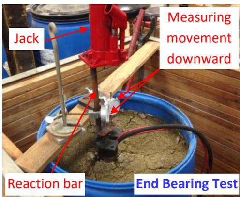
Figure 11 Setup of the end bearing loading test
