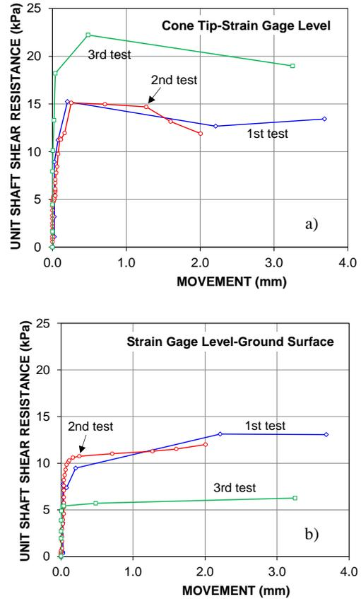
Figure 16 The unit shaft resistance-movement curves of bidirectional tests
