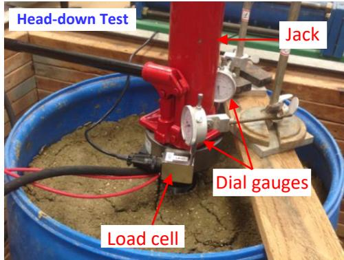
Figure 9 Setup of head-down loading test
