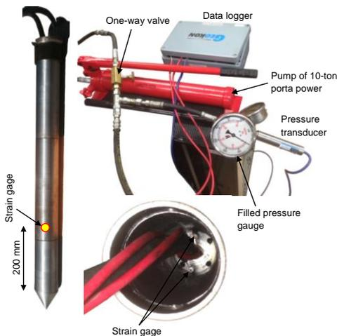
Figure 4 The Prototype P-cone device
