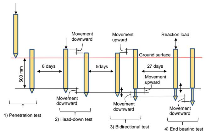
Figure 8 Test procedure of the P-cone performed
