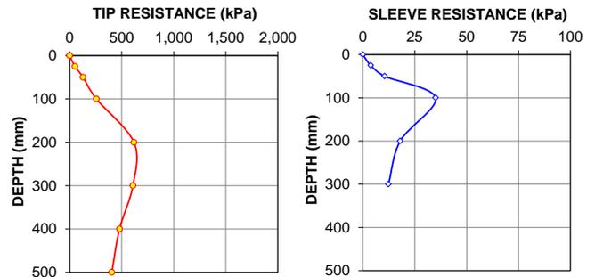
Figure 12 Shaft and tip resistance during P-cone penetration
