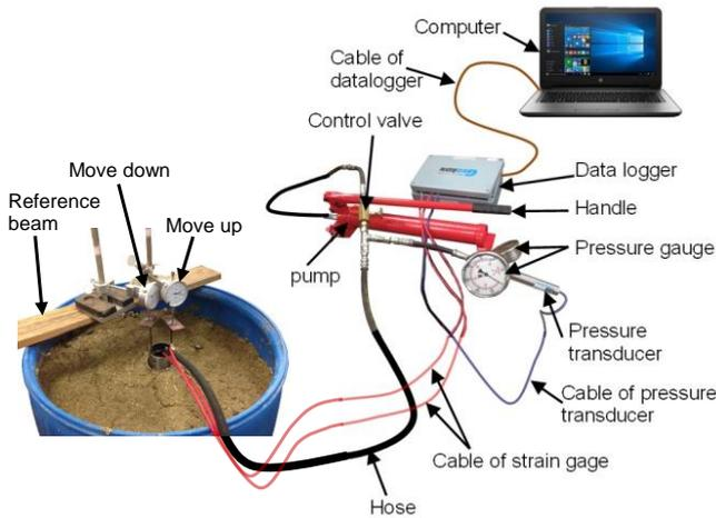
Figure 6 The bidirectional load test and the measurements operating principle and the measurement system of the P-Cone.
