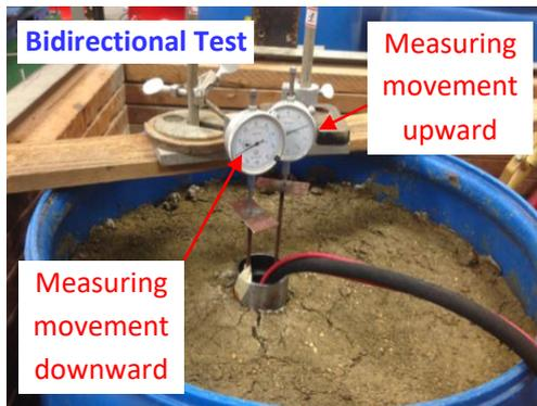
Figure 10 Setup of bidirectional loading test
