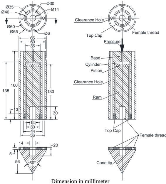
Figure 3 Detailed design of P-cone device
