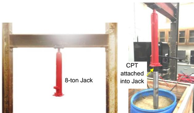
Figure 7 Jack attached to steel frame as reaction system
