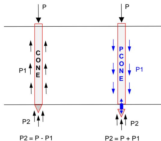
Figure 1 Illustration of the penetrating depth improvement
