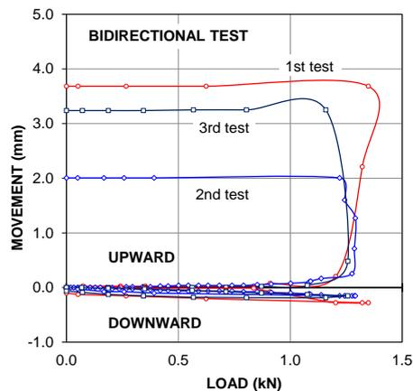
Figure 15 Load-movement curves of bidirectional loading tests
