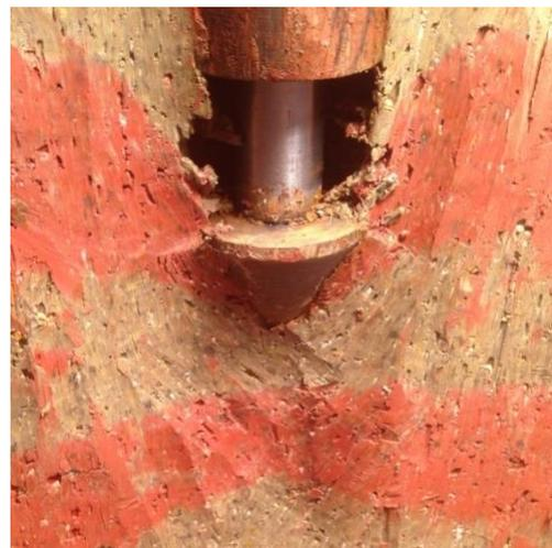
Figure 19 Failure shape of soil below cone tip
