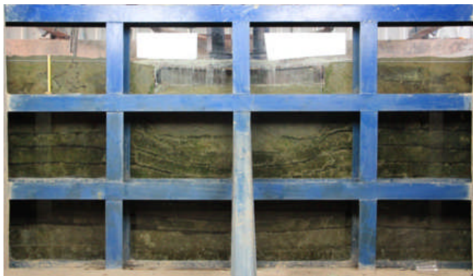
Figure 12 Displacement of ground without reinforcement that marked with sawdust
