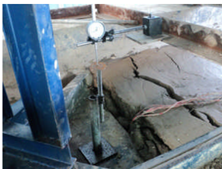
Figure 9 Devices measuring of installation settlement
