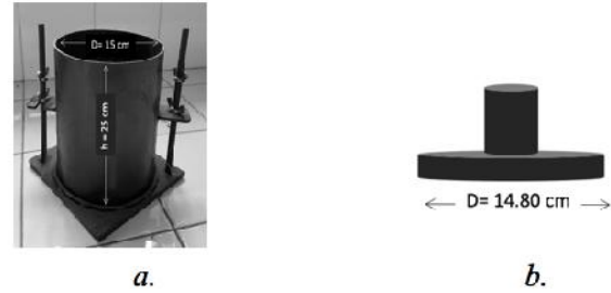
Figure 3 Compaction apparatus test: a. Cylindrical mould test; b. Anvil
