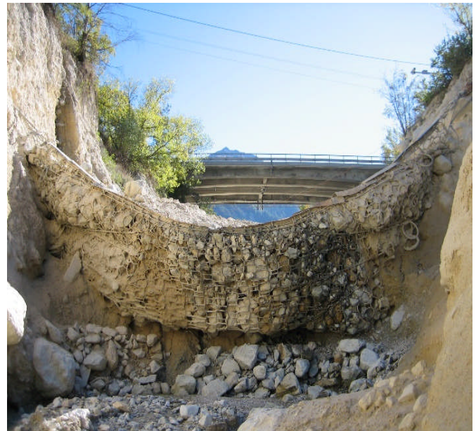
Figure 1 Testing of debris flow retention system with ring net in the Illgraben channel, 2006. Retention volume approx. 1000 m 3
