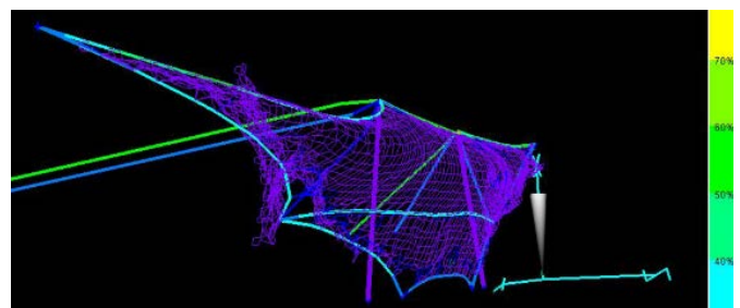
Figure 9 FARO simulation software output when barrier number 2 is impacted by an avalanche in Hasliberg, Switzerland
