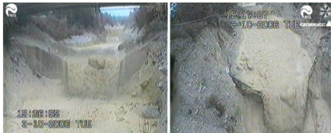
Figure 3 Large block (left) flowing over the balance and afterwards over the barrier (right)
