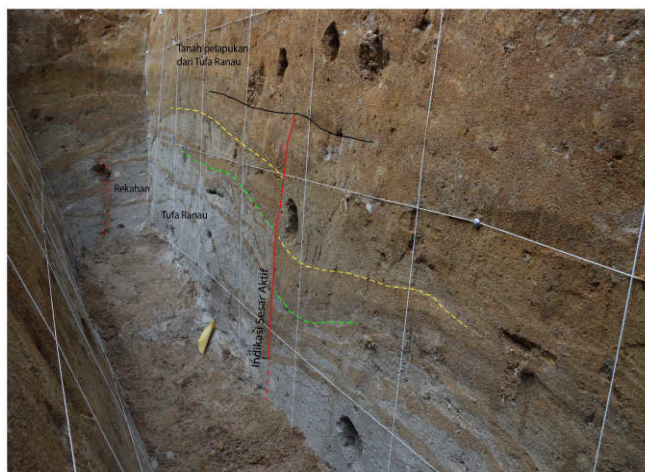
Figure 8. Indication of Pauh fault on the palaeoseismic trench wall
