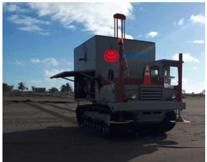
Figure 17 CPT rig with 20 ton capacity and auto-generated result
