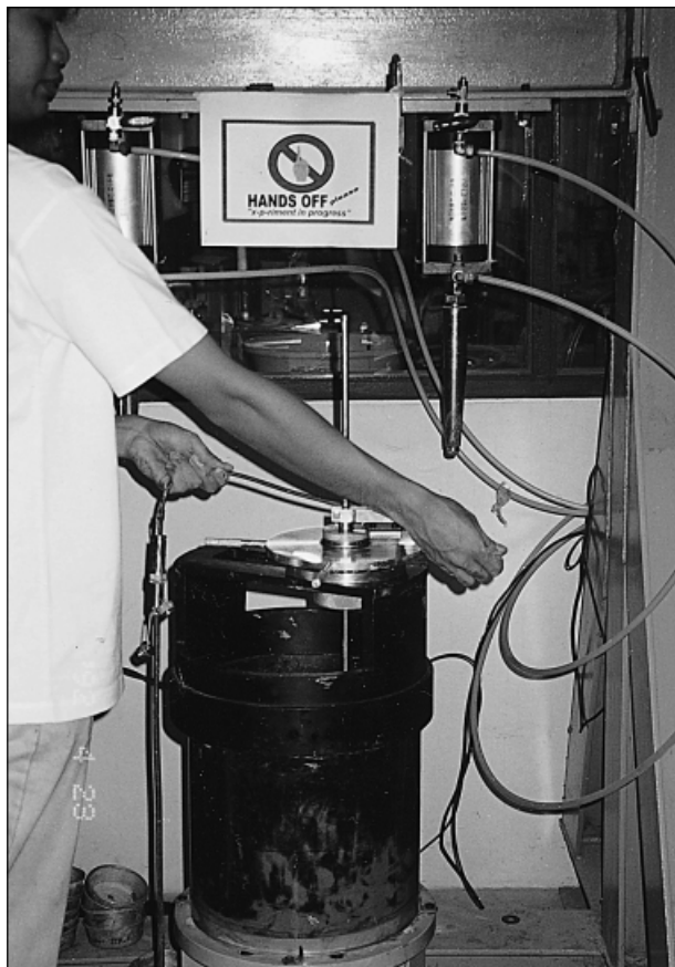
Fig. 5. Shear strength measurement using laboratory vane shear on the small electro-osmotic cylinder
