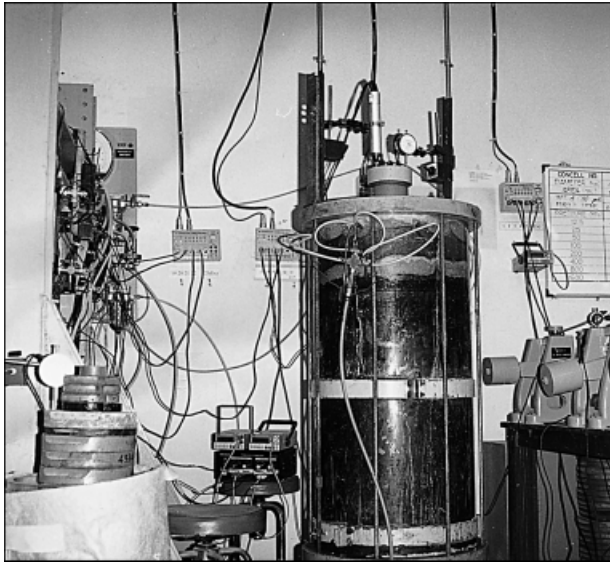
Fig. 4. Large consolidometer experimental set-up
