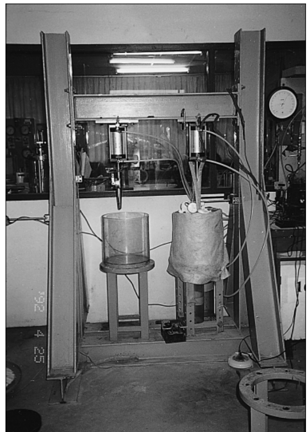
Fig. 3. Small electro-osmotic cylinder experimental set-up
