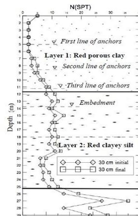
Figure 3 Typical profile of the SPT of the site
