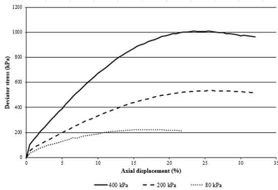
Figure 4a Deviator stress x Axial strain - 6m (Ruge, 2014)
