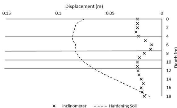
Figure 18 Horizontal displacements values - Hardening soil model
