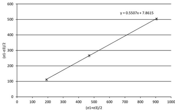
Figure 4b Shear stress x Effective normal stress - 6m (Ruge, 2014)
