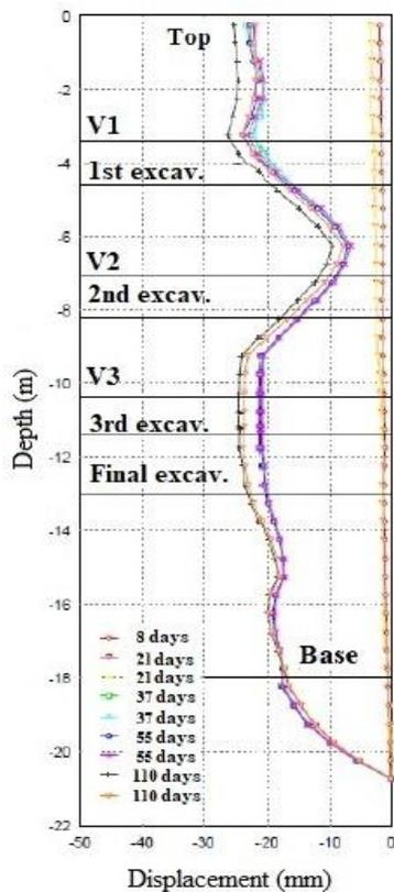
Figure 12 Results of the inclinometer (Ruge, 2014)
