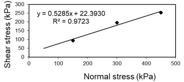
Figure 11 Direct shear test for 9m depth (Ruge, 2014)
