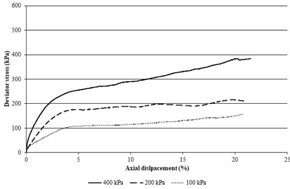
Figure 7 Undrained triaxial test for 6m depth
