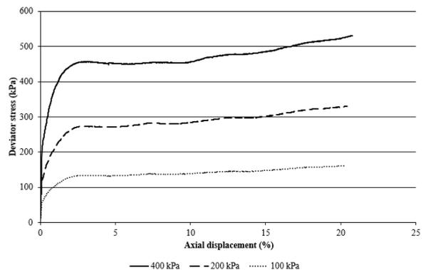
Figure 6 Undrained triaxial test for 3m depth
