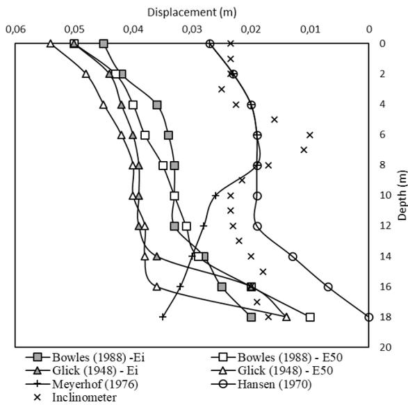
Figure 15 Horizontal displacements values of the pile curtain wall on the Sheeting Check software
