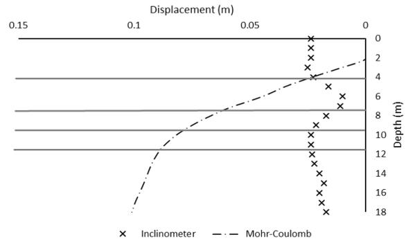
Figure 16 Horizontal displacements values - Mohr-Coulomb model
