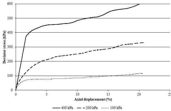
Figure 8 Undrained triaxial test for 9m depth (Ruge, 2014)
