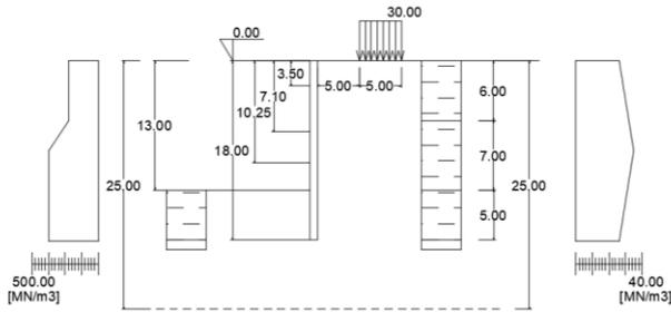
Figure 13 Ultimate stage of construction for Sheet Pile Check simulation
