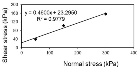
Figure 10 Direct shear test for 6m depth (Ruge, 2014)
