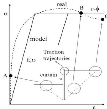
Figure 17 Stress-strain points on a typical soil behavior curve (Ruge, 2014)
