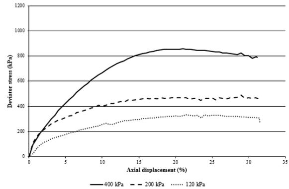
Figure 5a Deviator stress x Axial strain - 9m (Ruge, 2014)
