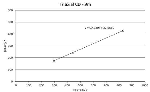
Figure 5b Shear stress x Effective normal stress - 9m (Ruge, 2014)
