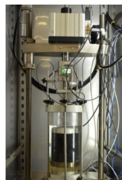
Dynamic creep test setup in wet condition (After Chompoorat and Likitlersuang, 2015)
