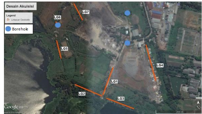
Figure 3. Locations of bore holes and resistivity measurements
