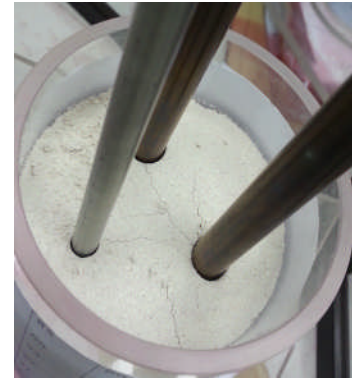
Figure 3 Soil sample after vibration process with fracture
