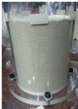
Figure 1 The prepared double-porosity soil
