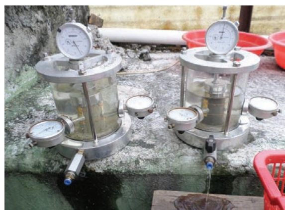
Figure 3. Three dimension (3D) of undisturbed sample volume changes device in wetting-drying process (Alatas I. M. 2017).
