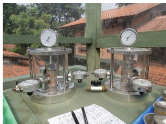
Figure 2. Three dimension (3D) of undisturbed sample volume changes device in drying process (Alatas I. M. 2017).
