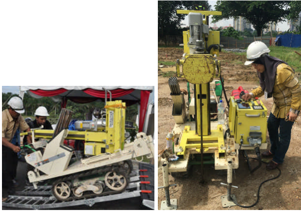
Figure 6 Screw Driving Sounding test at Setapak site
