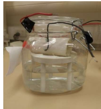
Figure 1 Test setup in the desiccator with different concentrations of NaCl solutions
