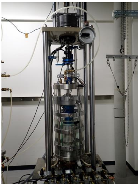
Photo 2: Triaxial cell of hollow cylinder torsional shear apparatus (After Toyota, Le and Takada, 2019)
