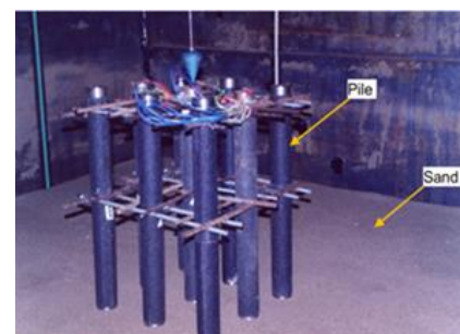
Bearing Capacity and Settlement Study on Small-Scale Piled-Raft Groups in Sand:
