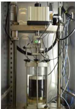
Dynamic creep test setup in wet condition (After Chompoorat and Likitlersuang, 2015)
