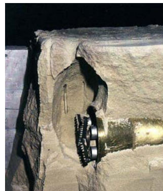
Unsupported cavity (After König et al., 2014)
