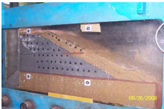
View of a soil confined coal ash embankment (After Viswanadham & Mathur, 2014)
