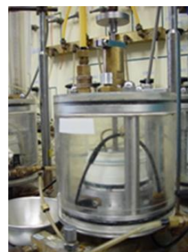
(b) View of the consolidation cell
