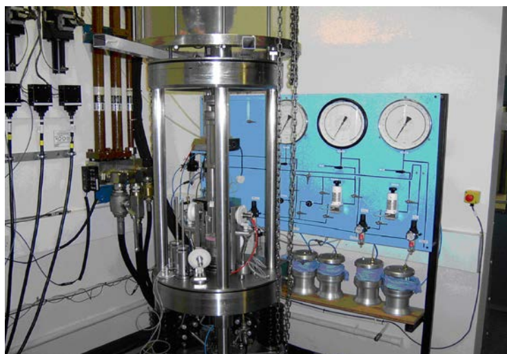
Hollow Cylindrical Torsional Apparatus (after Ibraim et al. , 2011)
