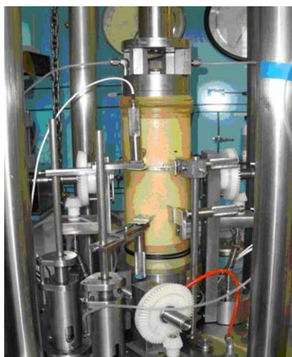
Local small strain measurement systems (after Ibraim et al. , 2011)
