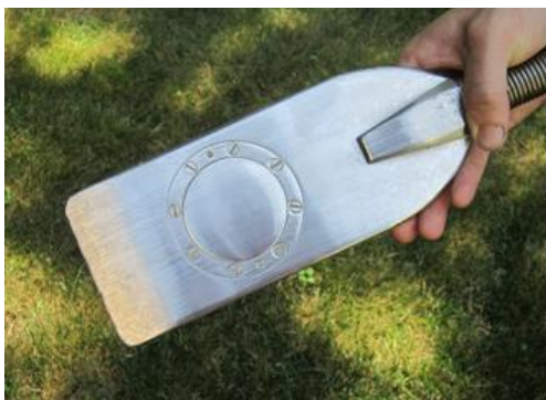
Dilatometer Earth Pressure Cell (after Lutenegeger, 2012)
