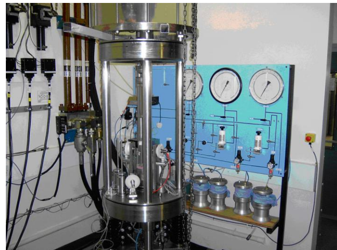
Hollow Cylindrical Torsional Apparatus (after Ibraim et al. , 2011)
