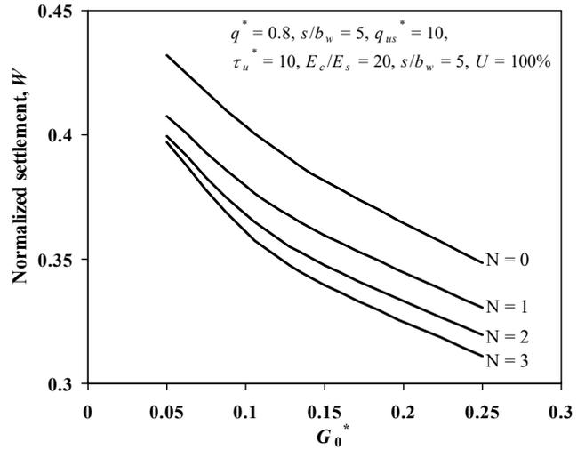
Figure 19 Effect of shear modulus of granular layer on normalized settlement at the centre of beam
