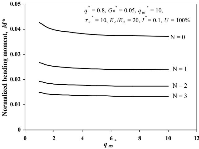
Figure 17 Effect of ultimate bearing capacity of soft soil on normalized bending moment at the centre of beam
