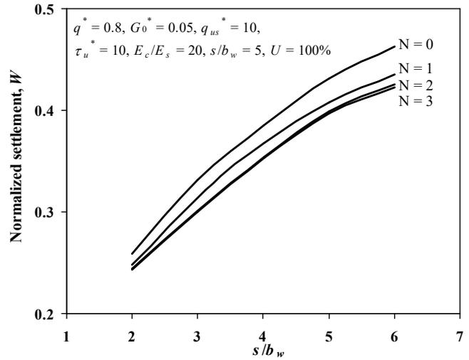
Figure 9 Effect of s/bw on normalized settlement at the centre of beam
