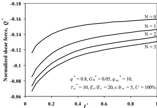
Figure 5 Effect of  $I^*$  on normalized shear force at the edge of the stone column
