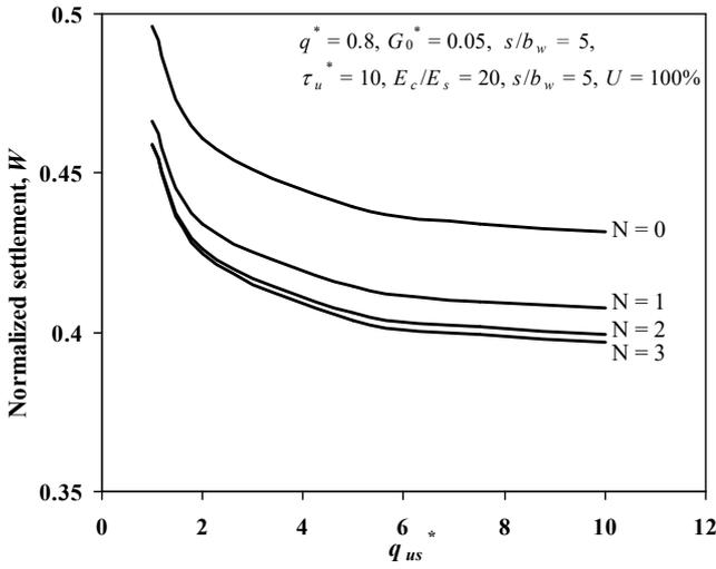
Figure 16 Effect of ultimate bearing capacity of soft soil on normalized settlement at the centre of beam
