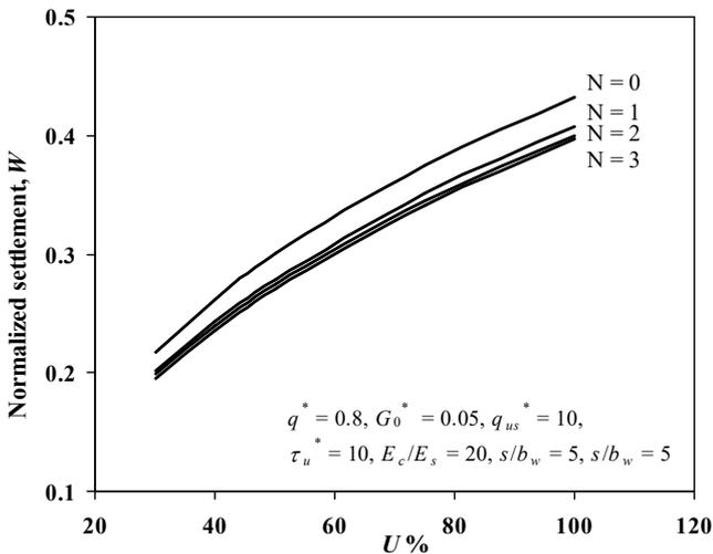
Figure 13 Effect of degree of consolidation on normalized settlement at the centre of beam
