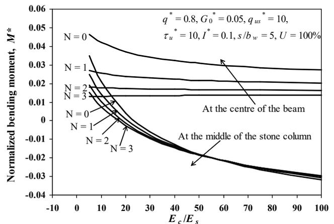
Figure 7 Effect of modular ratio on normalized bending moment
