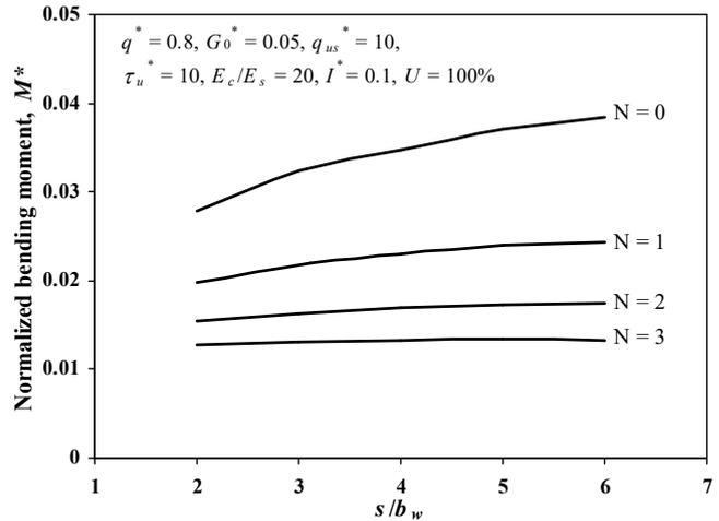
Figure 10 Effect of s/bw on normalized bending moment at the centre of beam
