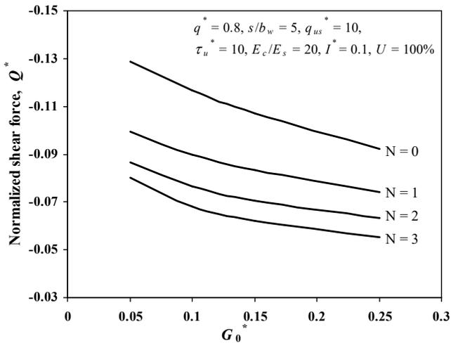
Figure 21 Effect of shear modulus of granular layer on normalized shear force at the edge of the stone column
