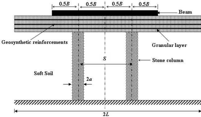
Figure 1 Beam resting on multilayered geosynthetic-reinforced granular fill on stone column-improved soft soil
