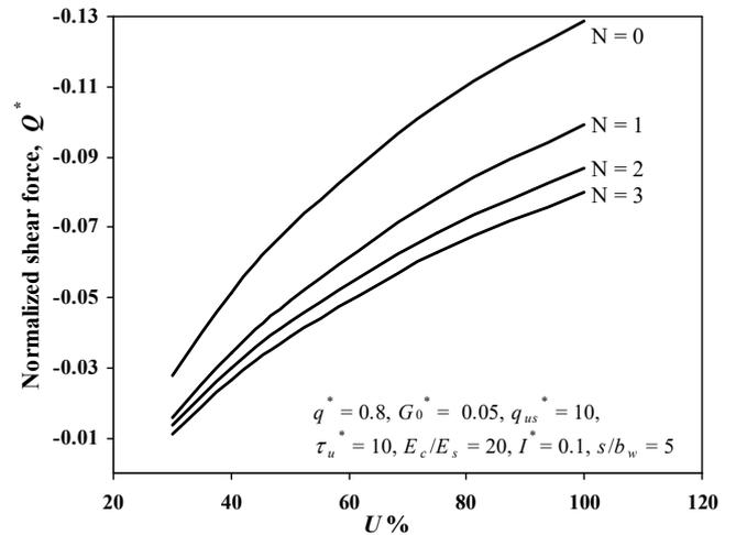
Figure 15 Effect of degree of consolidation on normalized shear force at the edge of the stone column
