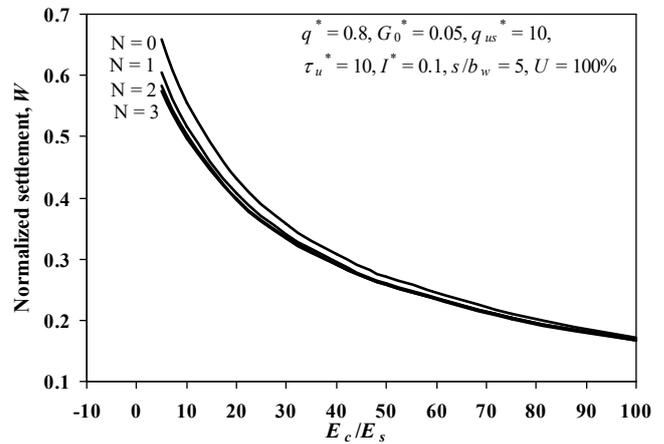
Figure 6 Effect of modular ratio on normalized settlement at the centre of beam
