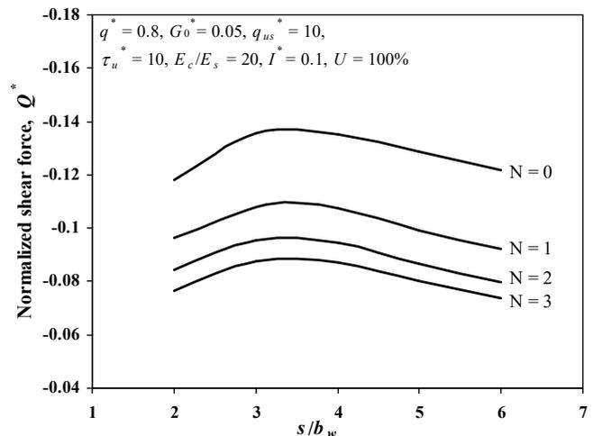
Figure 11 Effect of s/bw on normalized shear force at the edge of the stone column
