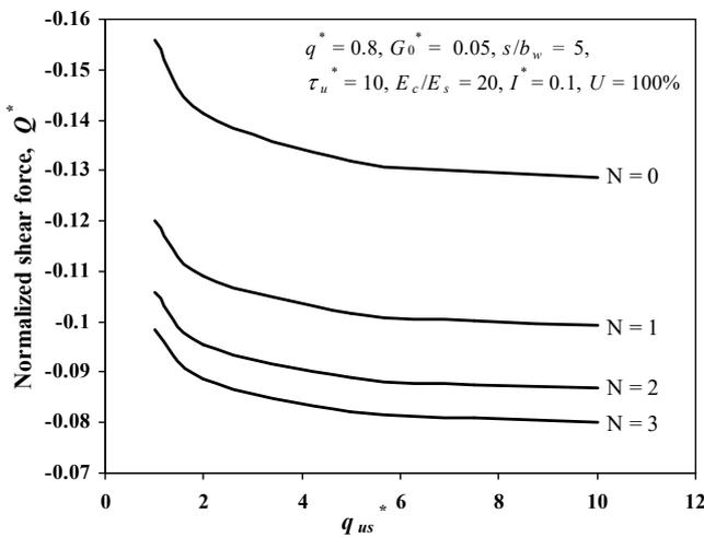
Figure 18 Effect of ultimate bearing capacity of soft soil on normalized shear force at the edge of the stone column
