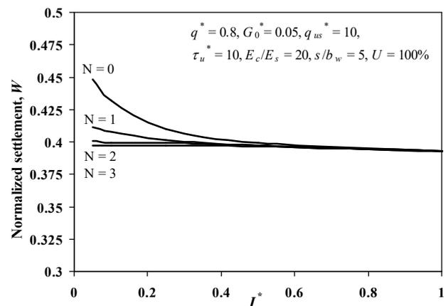
Figure 3 Effect of  $I^*$  on normalized settlement at the centre of beam
