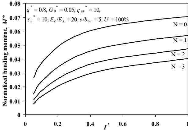
Figure 4 Effect of  $I^*$  on normalized bending moment at the centre of beam
