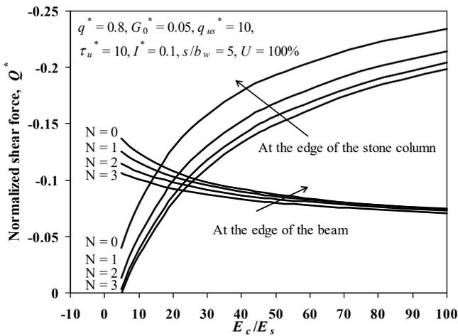
Figure 8 Effect of modular ratio on normalized shear force
