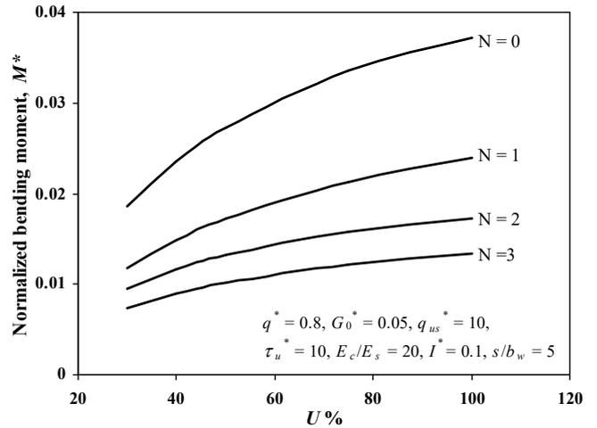
Figure 14 Effect of degree of consolidation on normalized bending moment at the centre of beam
