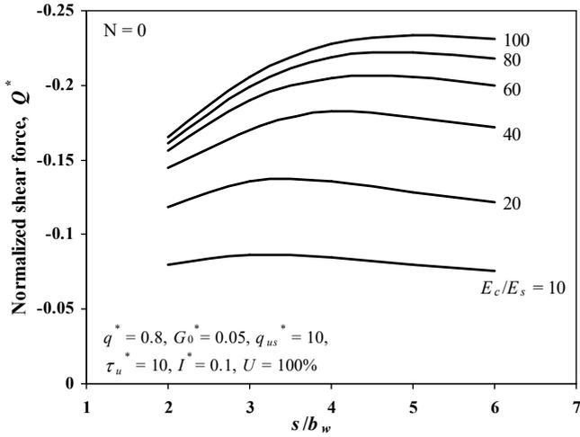
Figure 12 Variation of normalized shear force with  $s/b_w$  for different modular ratio values ( $N = 0$ )
