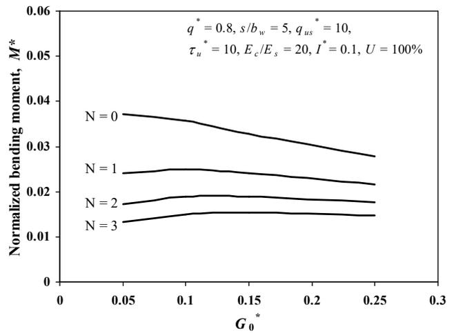
Figure 20 Effect of shear modulus of granular layer on normalized bending moment at the centre of beam
