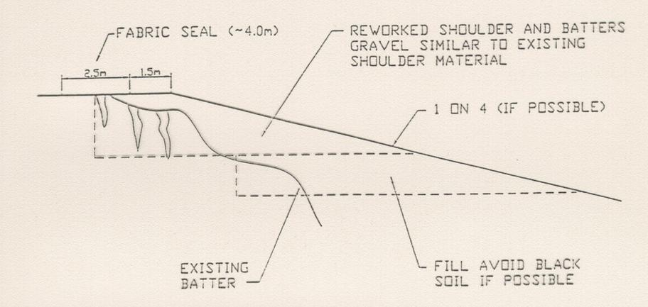
Figure 5 - Rehabilitation Treatment for Longitudinal Cracking
