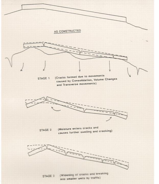
Figure 3 – Failure Mechanism
