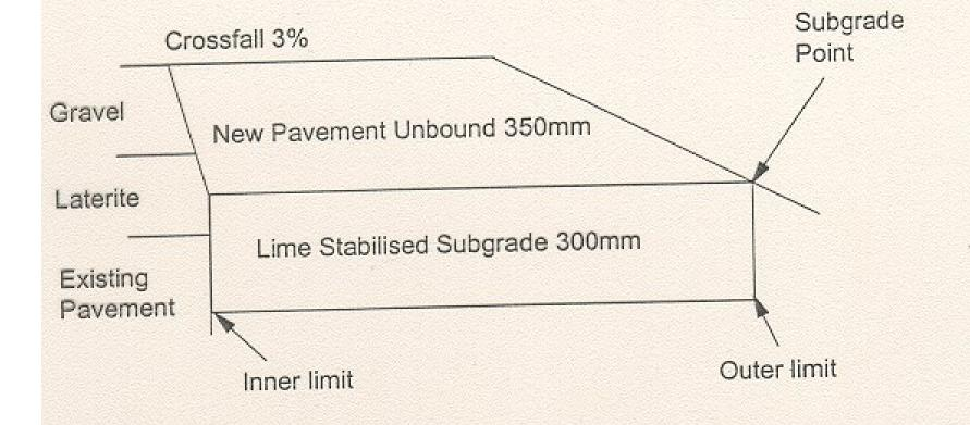
Figure 1- Lime Stabilisation of Expansive Soil Subgrade
