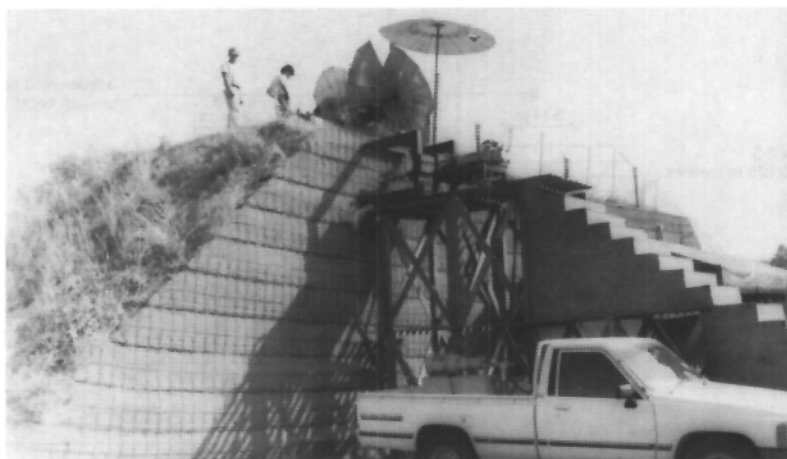
Fig. 11. Typical field pullout test set-up
