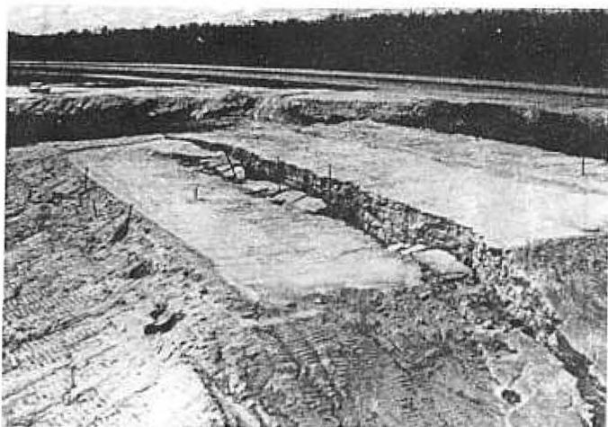
FIG. 2. View of Tensile Fracture of Compacted Fill
