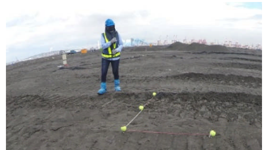
Figure 14. Images acquisition process of the initial site condition with its GCPs (Ground Control Points)
