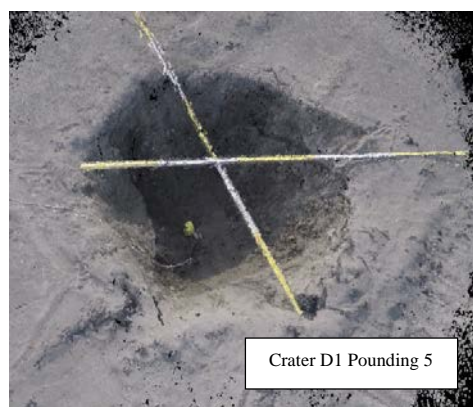
Figure 24. 3D model from point cloud data of a DC crater for different pounding (birds-eye view) (contd.)
