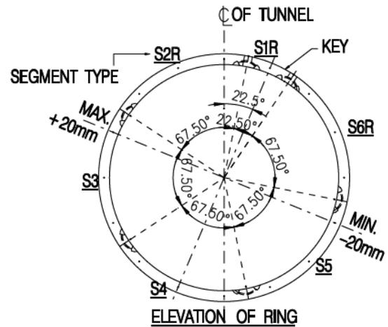
Figure 3 Typical general arrangement of segmental lining for CCL bored tunnels
