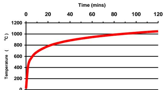
Figure 16 Fire curve specified in BS476-20:1987
