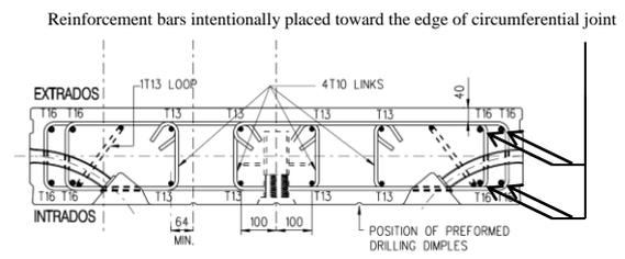
Figure 4 Detailing of steel bars at circumferential joints
