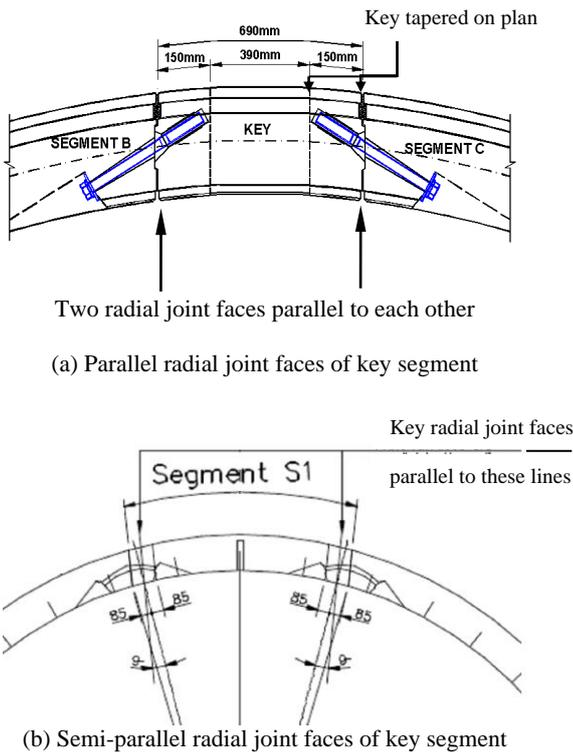
Figure 2 Examples of parallel and semi-parallel radial joint faces of key segment
