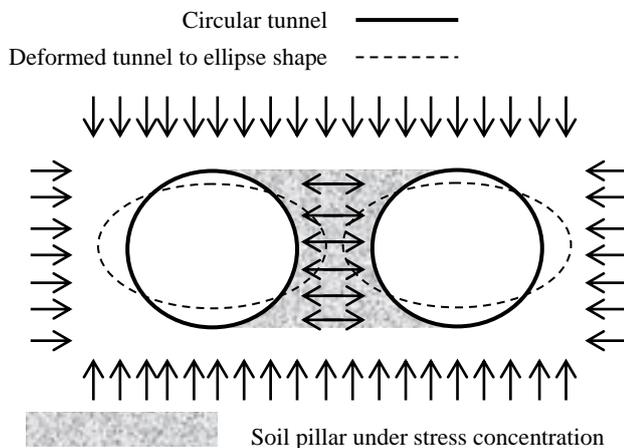
Figure 12 Stress concentrations at soil pillar between twin tunnels
