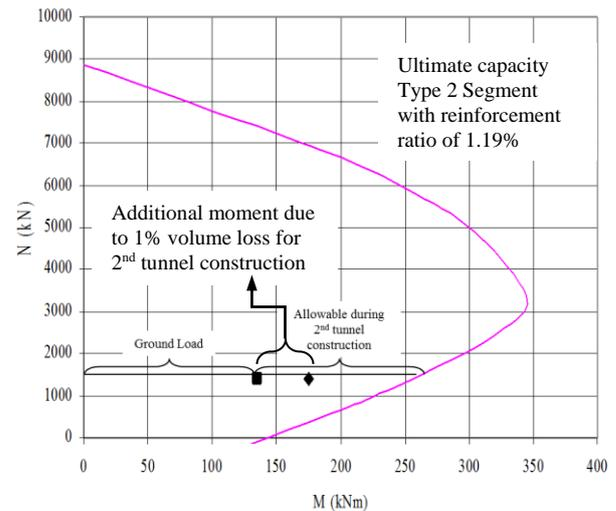
Figure 10 M-N interaction diagram for serviceability limit state (0.2mm crack width) and ultimate limit state
