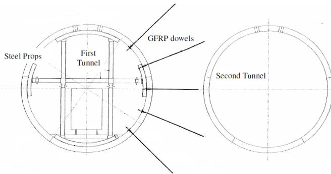
Figure 11 (a) Scheme of passive support and GFRP dowels for tunnels in close proximity (Lim, et al 2008)
