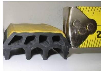
(b) Proposed co-extruded composite gasket in CCL
