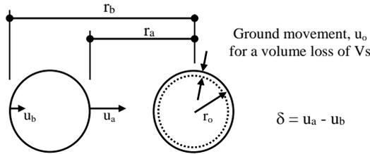
Figure 8 Distortion of first tunnel lining due to second tunnel construction in close proximity, Wen et al (2004).
