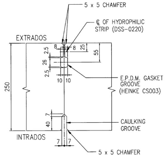
Figure 19 Typical gasket arrangements with hydrophilic strips and EPDM gaskets at extrados
