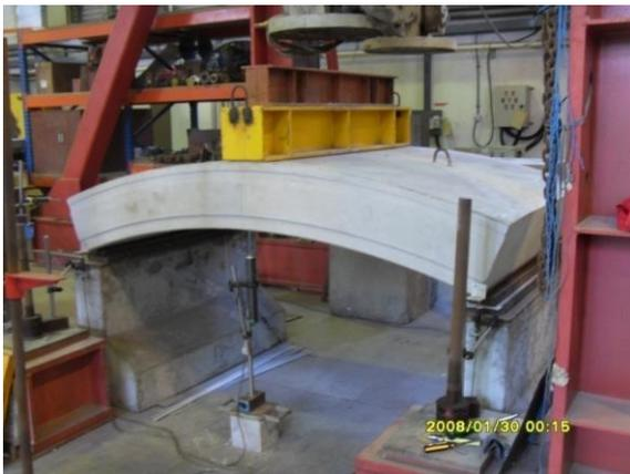
Figure 24 Full scale segment test to verify moment capacity of SFRC segments
