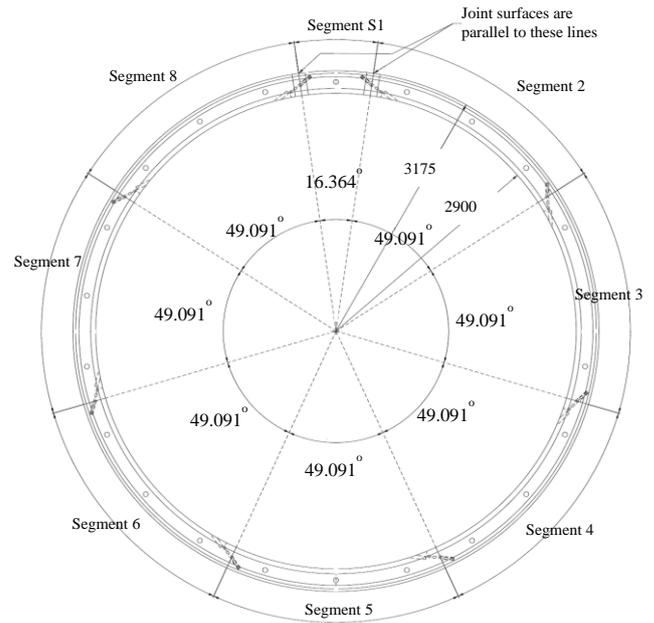
Figure 25 General arrangements of segments for DTL3 SFRC segmental lining
