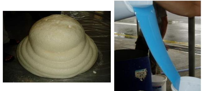
Figure 20 Water-reactive polyurethane grout forming open-cell foam (left) and flexible grout forming a membrane (right)
