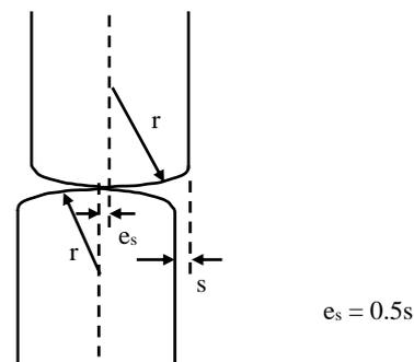
Figure 6 Eccentricity due to step across a double convex joint
