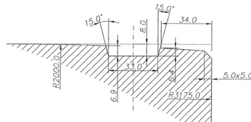
(c) Gasket groove for the composite gasket in CCL
