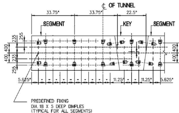
Figure 13 Pre-defined drilling locations (dimples) on the precast reinforced concrete segments since CCL MRT projects
