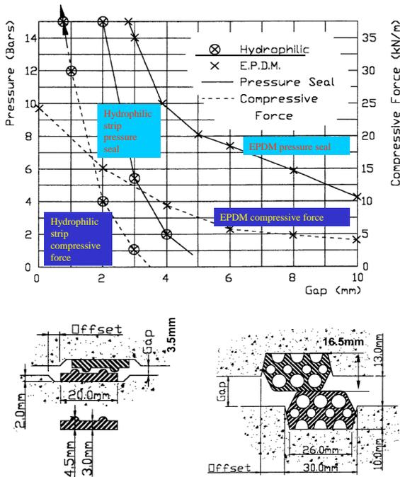
Figure 21 Sealing capacities of hydrophilic strip / EPDM vs. compression of strip, after Doran (1997)
