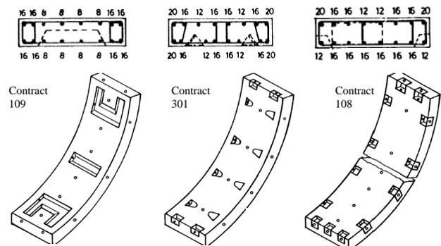
Figure 1 Typical segment used in Phase I/II MRT projects (Copsey & Doran, 1987)
