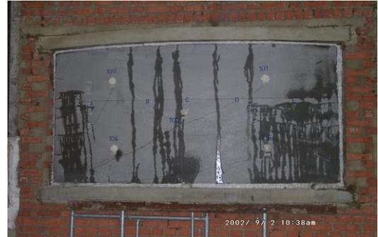
Figure 15 Fire testing of a partial segment specimen with extrados exposed and intrados facing the furnace under fire
