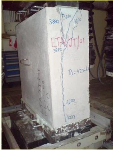
Figure 23 Full scale tests of segment joints under concentrated compression loading to simulate the hoop thrust at segment joints
