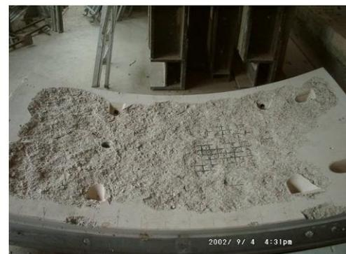
Figure 17 Concrete spalling up to the depth of wire mesh after fire test for the segment specimen
