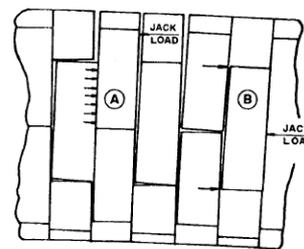
Figure 5 Segment under lateral bending due to installation inaccuracy during shoving of TBM (after Copsey & Doran, 1987)
