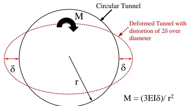
Where M is the additional moment due to distortion of 2δ of 15mm on diameter, or δ of 7.5mm on radius of r; E is the Young’s modulus and I the moment of inertia of the segment.
