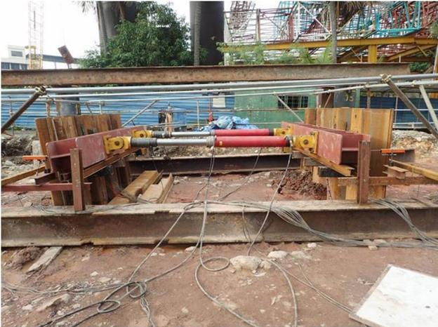
Figure 7 Lateral load test at maximum load (Case1: Left, IV-pile wall; Right, 25H-pile wall)
