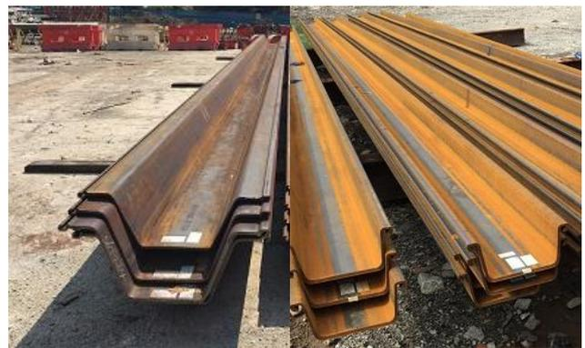
Figure 4 Test piles (Left: Hat-45H-pile, Right: IV-pile)
