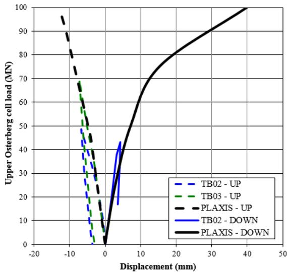
Figure 4 Measured versus predicted performance for loading at upper Osterberg cells
