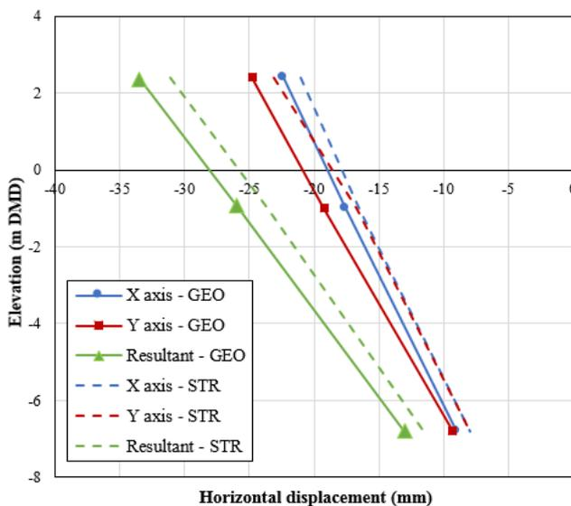
Figure 13 Comparison of calculated lateral displacements from geotechnical (GEO) and structural (STR) analyses
