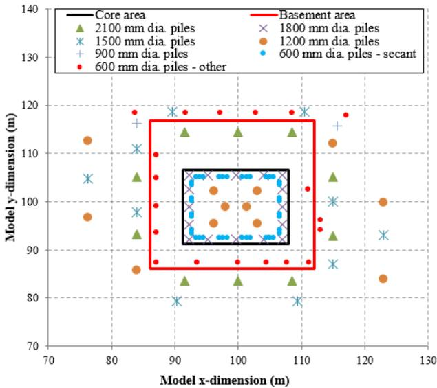
Figure 10 Pile layout of the foundation system
