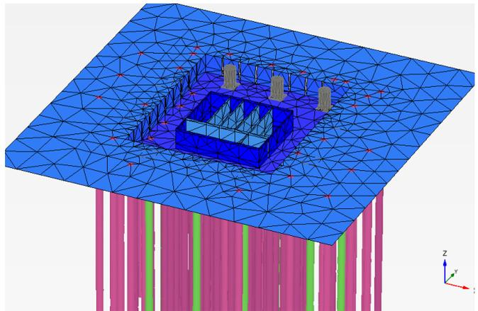
Figure 12 PLAXIS 3D model of stability system of Australia 108
