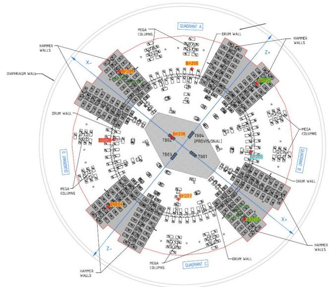
Figure 6 Plan view of footing layout
