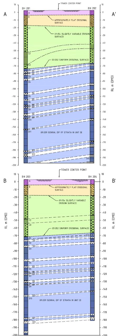
Figure 1 Orthogonal cross sections through the site showing general stratigraphy
