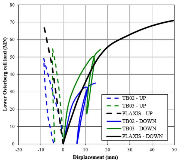
Figure 5 Measured versus predicted performance for loading at lower Osterberg cells
