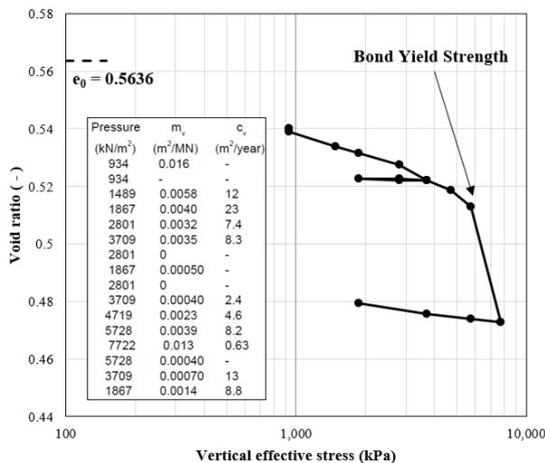
Figure 2 Results of oedometer test undertaken on sample recovered from 182.5 m with approximate Bond Yield Strength indicated
