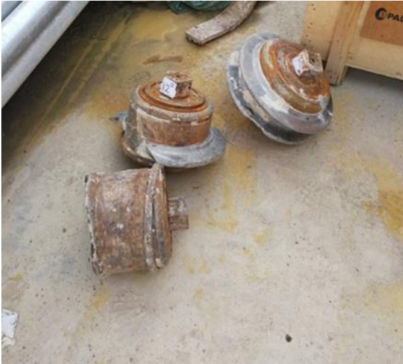
Figure 6 Abscission and eccentric wear of double edged disc in Karst stratum
