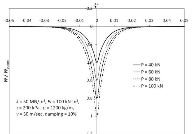
Figure 3 Deflection profile of geocell reinforcement: influence of applied load
