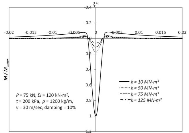
Figure 7 Variation in bending moment: influence of subgrade modulus of foundation soil
