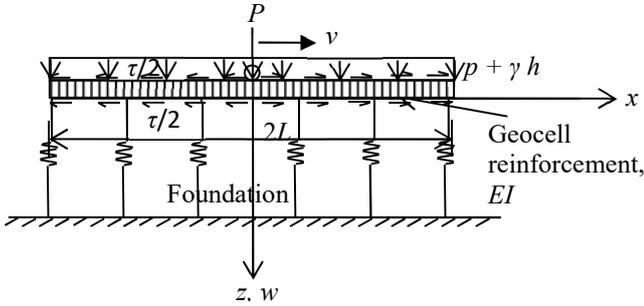
Figure 1 Schematic diagram and proposed model for geocell reinforced earth bed
