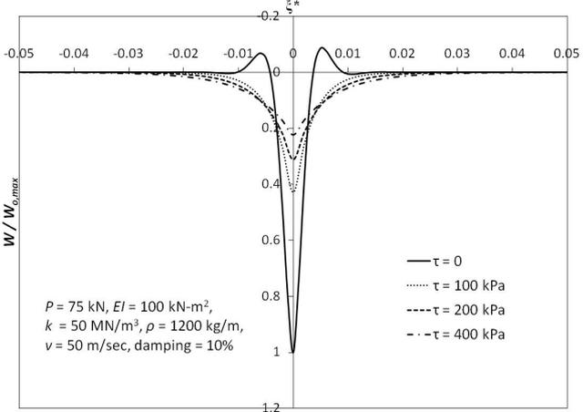
Figure 10 Deflection profile of geocell reinforcement: influence of interface resistance
