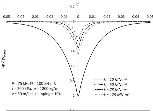
Figure 6 Deflection profile of geocell reinforcement: influence of modulus of subgrade reaction
