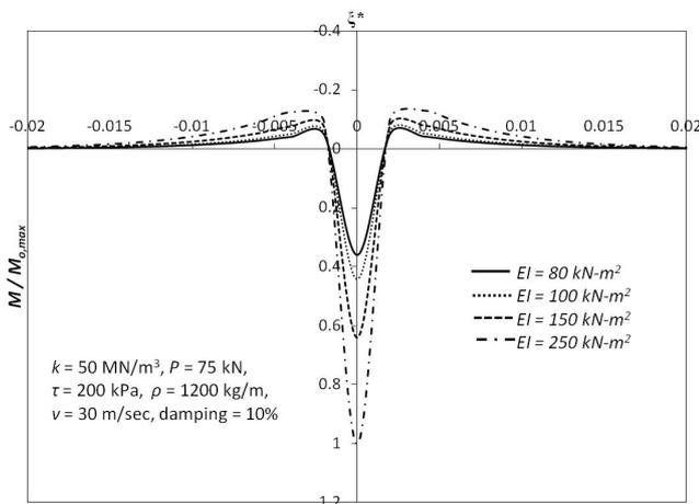
Figure 5 Variation in bending moment: influence of flexural rigidity of geocell reinforcement
