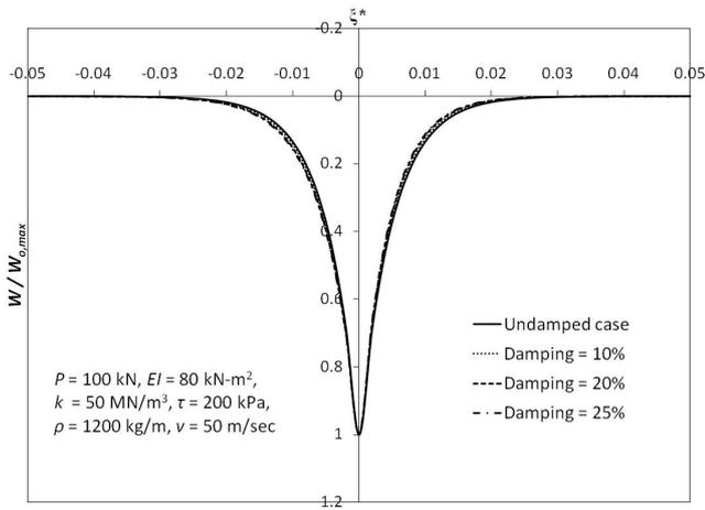
Figure 8 Deflection profile of geocell reinforcement: influence of damping
