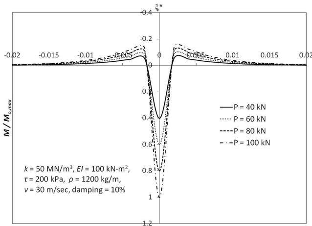
Figure 4 Variation in bending moment: influence of applied load
