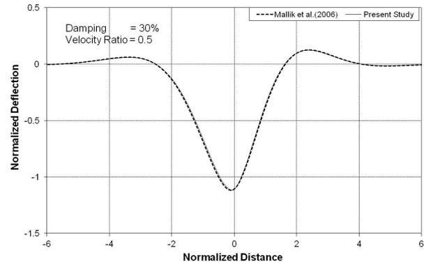
Figure 2 Comparison of deflection profile of geocell with Mallik et al. (2006)
