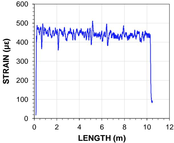
Figure 5 Pre-tension strain of a FO strain cable
