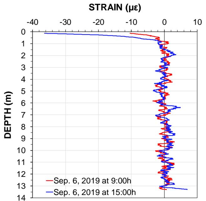
Figure 13 An example of the influence of daily ground temperature changes on the individual FO strain cable on Sep. 6, 2018 from an initial reading taken the same day at 06:30h
