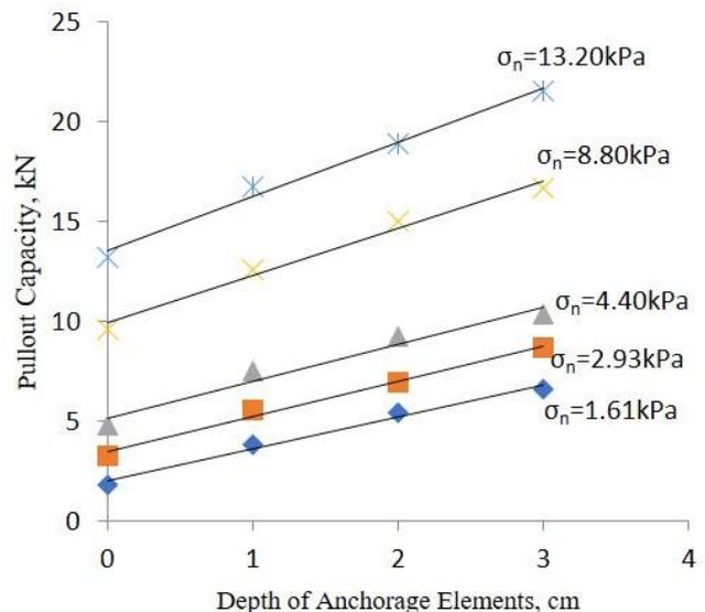
Figure 12 Pullout capacities versus depths of anchorage elements for strips under various normal stresses
