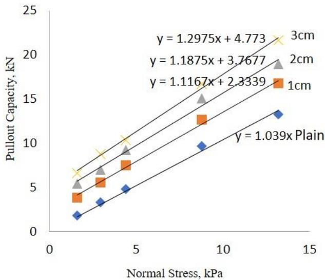
Figure 13 Pullout capacities versus normal stresses for various strips
