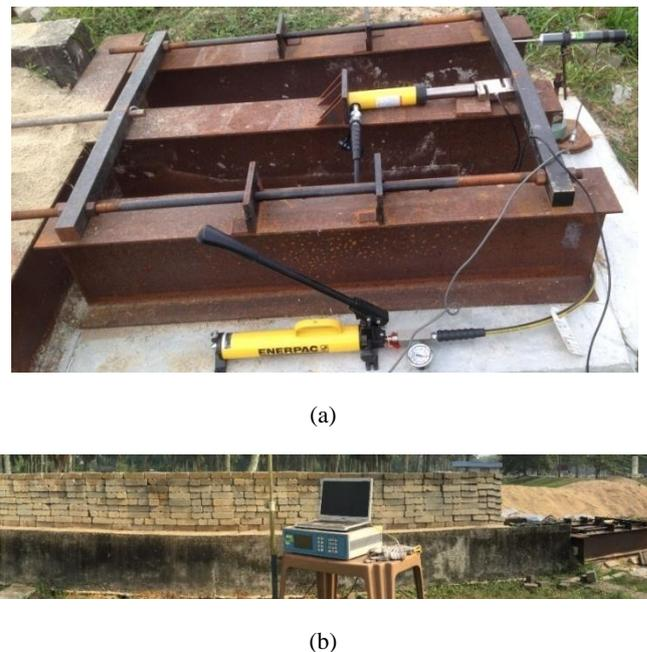
Figure 7 Photos of pullout test apparatuses (a) Pullout assembly consisting of pulling rod, pullout frame, hydraulic jack, load cell, LVD transducer, pedestal, reaction beam, and concrete base (b) Overall assembly consisting of compartment walls, layers of bricks, data logger, laptop computer, and the pullout assembly
