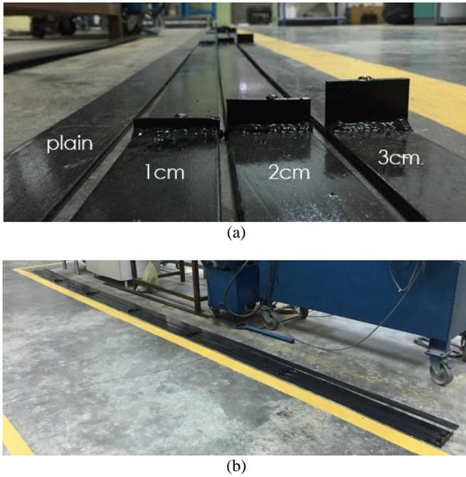
Figure 5 Photos of plain strip and strips with anchorage elements of 1cm, 2cm, and 3cm respectively (a) Front view (b) Oblique view
