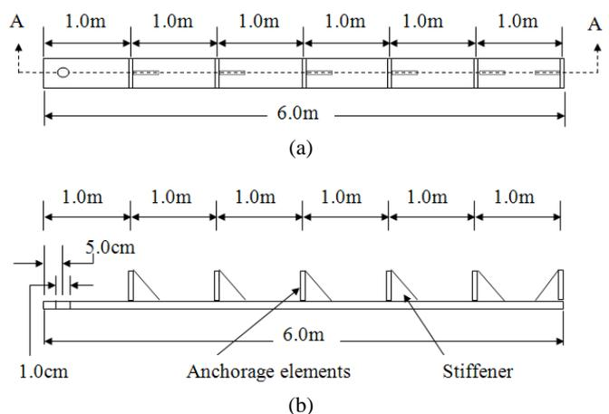
Figure 4 Views of a strip with anchorage elements and stiffeners (a) Plan view (b) Side view through Section A-A
