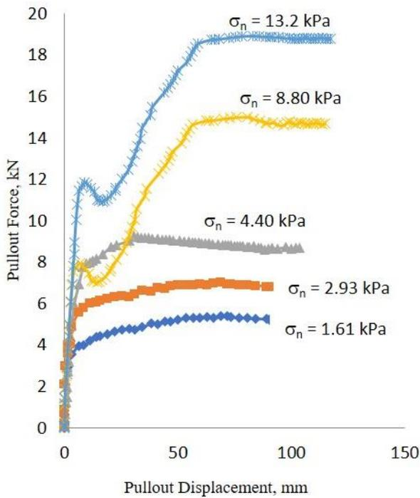
Figure 10 Pull-out forces versus displacements for strip with anchorage elements of 2cm depth under various normal stresses
