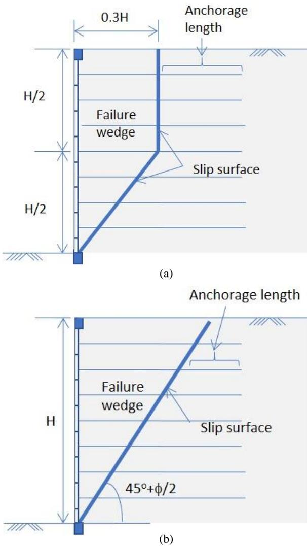
Figure 2 Conceptual slip surfaces of the MSE (a) Case of inextensible strip (b) Case of extensible strip (Salgado, 2008)
