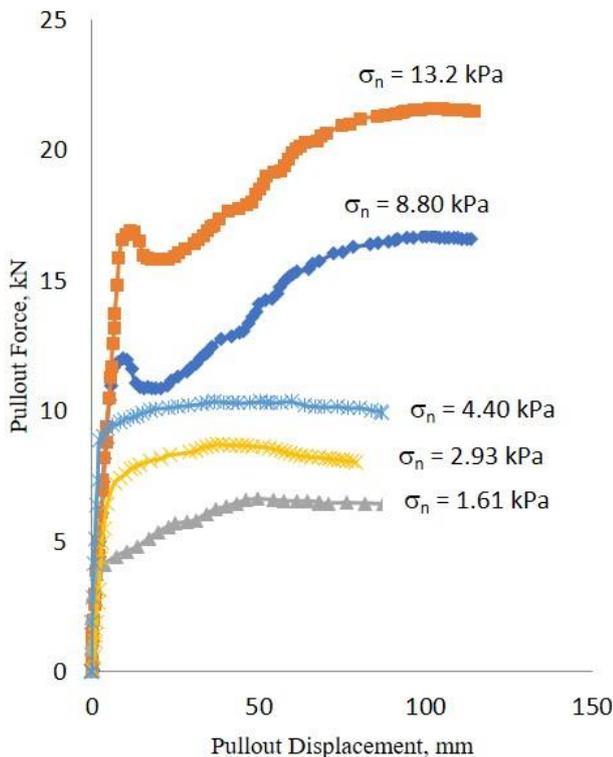
Figure 11 Pull-out forces versus displacements for strip with anchorage elements of 3cm depth under various normal stresses
