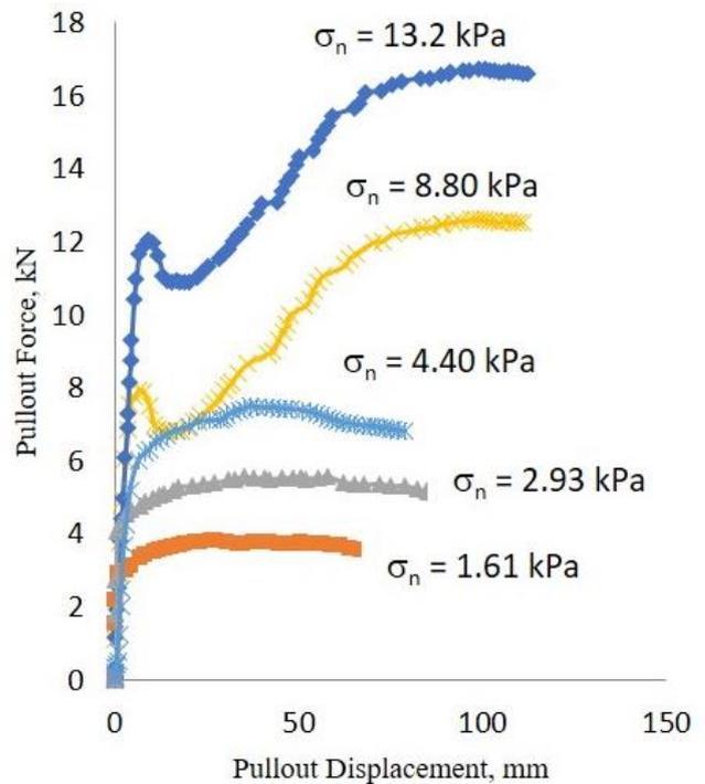
Figure 9 Pull-out forces versus displacements for strip with anchorage elements of 1cm deep under various normal stresses
