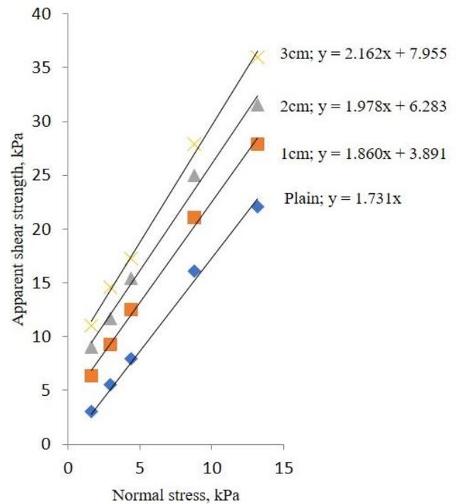
Figure 14 Normal stress versus apparent shear strength
