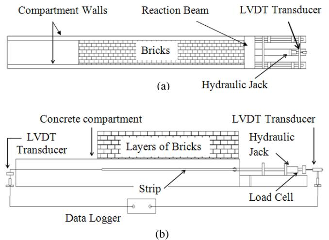
Figure 6 Schematic diagram of field pull out test apparatus (a) Plan view (b) Side view
