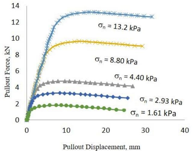
Figure 8 Pull-out forces versus displacements for plain strip under various normal stresses
