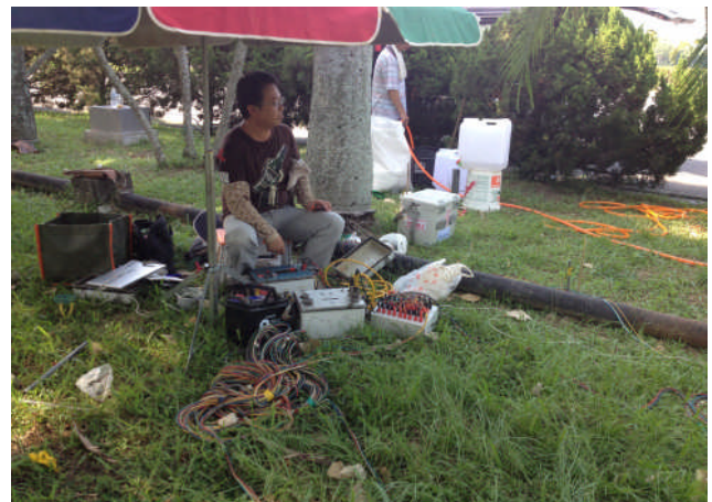
Figure 17 ERT-based brine tracing conducted at borehole WH-3
