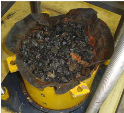
(c) Test with geotextile GT2 (SS test)
