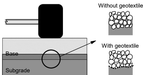
Figure 1 Geotextile separation mechanism
