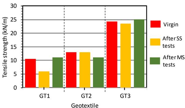
Figure 13 Geotextile tensile strength before and after the tests
