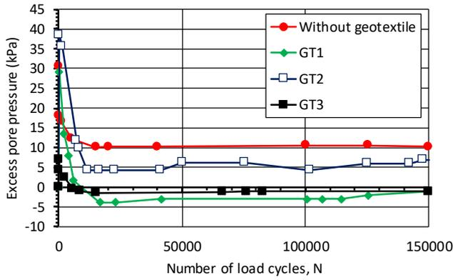
Figure 8 Excess pore pressure at piezometer P2 versus number of load cycles – SS tests
