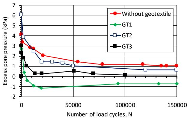
Figure 5 Excess pore pressure at piezometer P1 versus number of load cycles – MS tests
