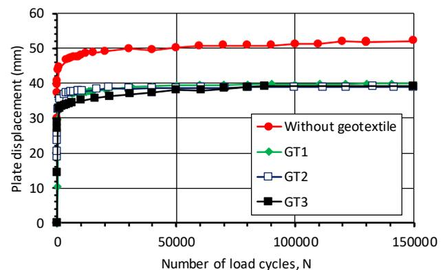
Figure 4 Plate settlement versus number of load cycles – SS tests
