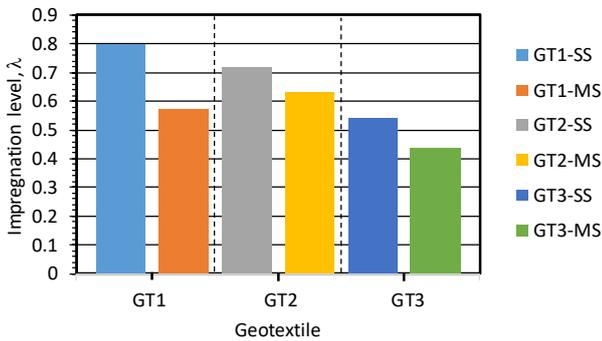
Figure 9 Impregnation levels of the geotextiles
