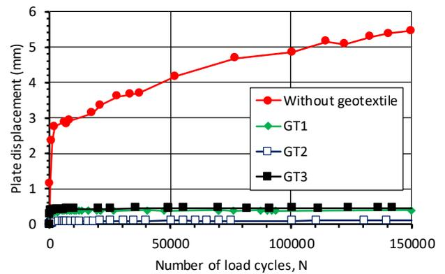
Figure 3 Plate settlement versus number of load cycles – MS tests
