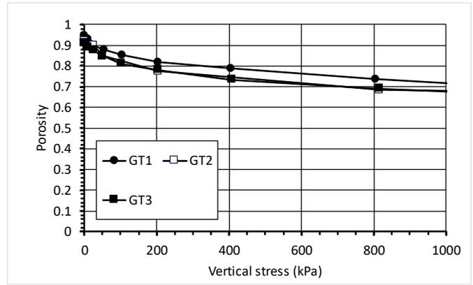
Figure 10 Geotextile porosity versus vertical stress
