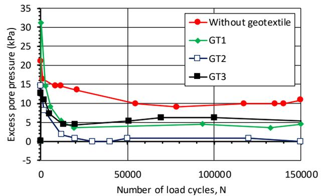
Figure 6 Excess pore pressure at piezometer P2 versus number of load cycles – MS tests
