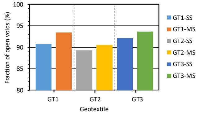
Figure 11 Geotextile fraction of open voids
