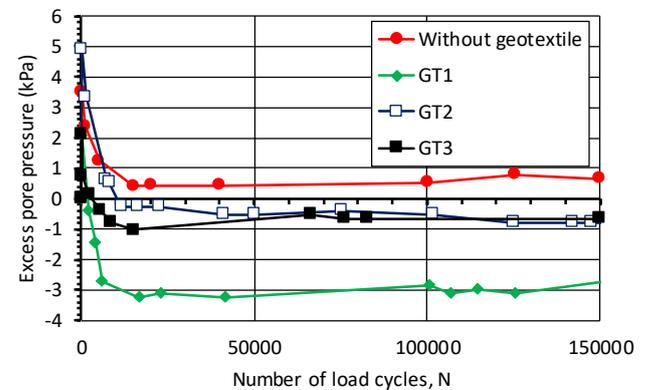
Figure 7 Excess pore pressure at piezometer P1 versus number of load cycles – SS tests
