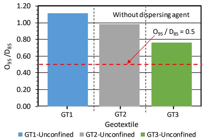
(a) For unconfined geotextile conditions
