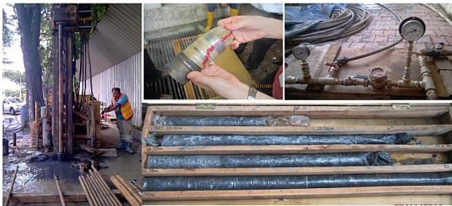
Figure 7 Photos of obtaining Undisturbed Samples with double tube with plastic liner.
