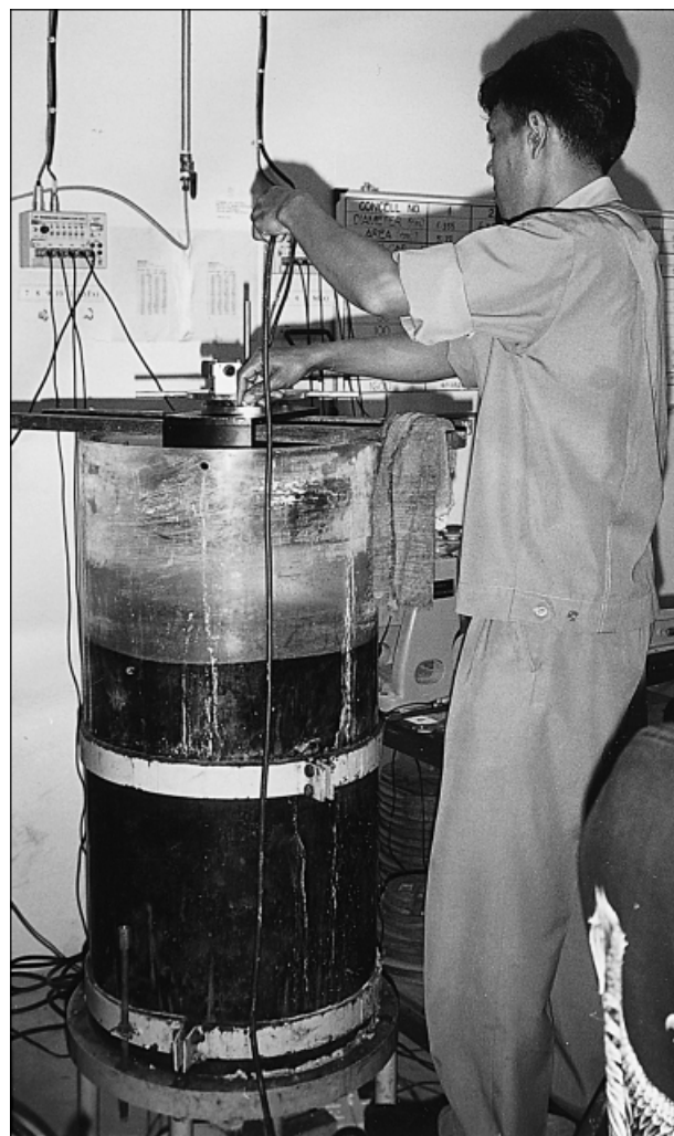
Fig. 6. Shear strength measurement using laboratory vane shear on the large consolidometer
