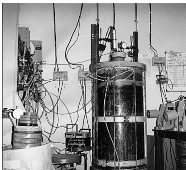
Fig. 4. Large consolidometer experimental set-up
