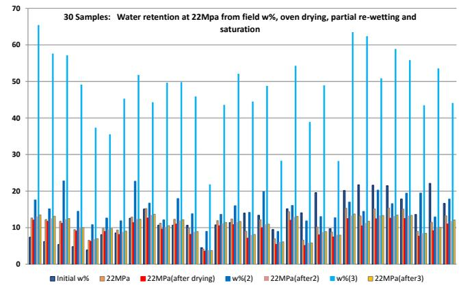
Figure 6 Water content reached by 30 samples at 22MPa from initial moisture content, after oven drying, after wetting and after saturation
