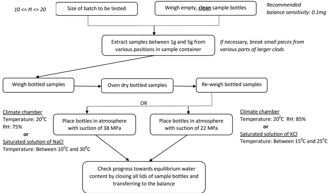
Figure 24 Flow Chart showing the Procedure of a balance between speeds, simplicity, ease of preparation, economy of apparatus and reliability of results
