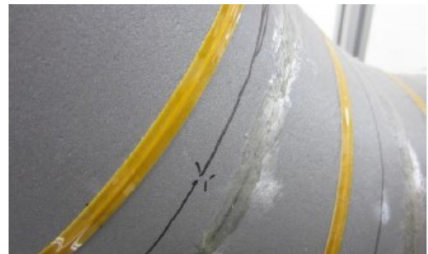
Figure 13 Application of a tape sensing fiber spirally adhered to a steel pipe for detecting strain (courtesy of Neubrex)
