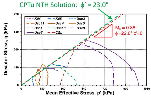
Figure 7 Triaxial tests on Speswhite kaolin clay (data from Valls-Marquez 2009)
