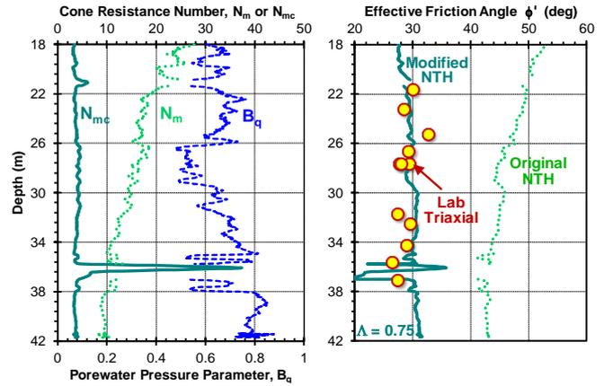
Figure 11 Profiles at Anchorage: (a) normalized CPTu parameters; (b) interpreted  $\phi'$  from triaxial tests and CPTu using NTH solution
