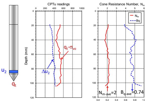
Figure 5 Miniature CPTu in calibration chamber of NC kaolin (data from Hird & Sangtian 2003)
