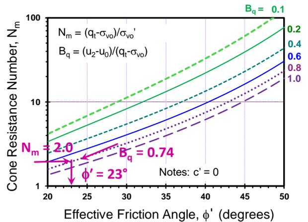
Figure 6 Evaluation of  $\phi'$  for Speswhite kaolin in chamber test
