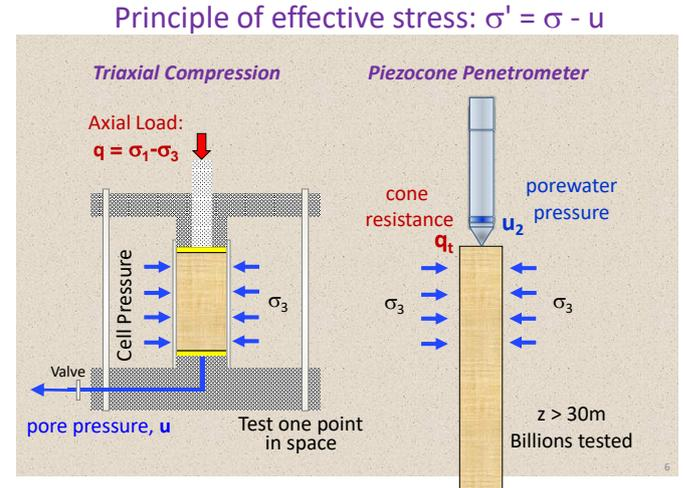
Figure 4 Conceptual comparison between triaxial apparatus and the piezocone penetrometer
