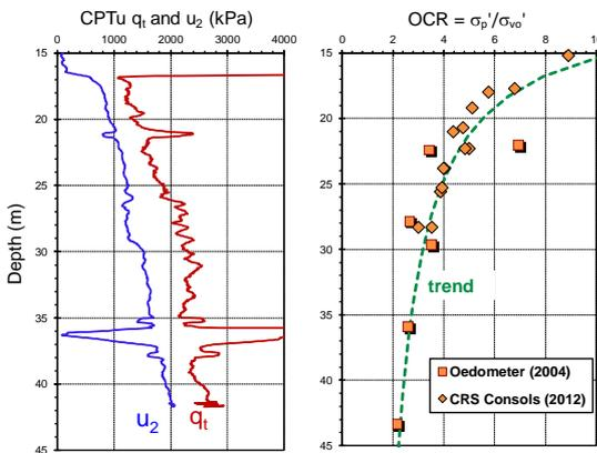
Figure 9 Representative profiles at Port of Anchorage: (a) CPTu results; (b) overconsolidation ratio from lab consolidation tests (data from Mayne & Pearce 2005)
