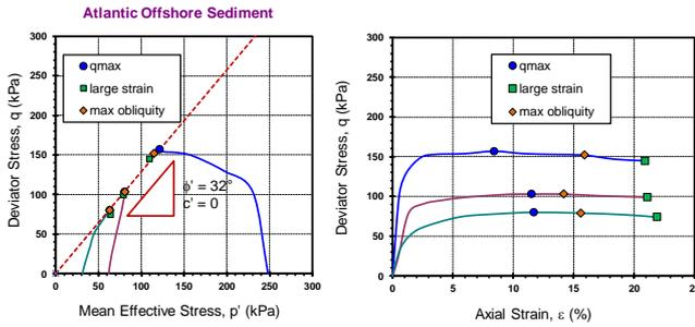
Figure 3 Comparison of three criteria for defining magnitude of  $\phi'$  for an Atlantic offshore sediment from triaxial test results (data from Olsen et al. 1986)
