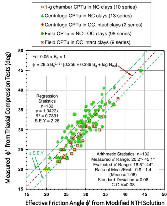
Figure 12 Summary plot of laboratory triaxial measured  $\phi'$  versus CPTu  $\phi'$  from different test series using modified NTH method
