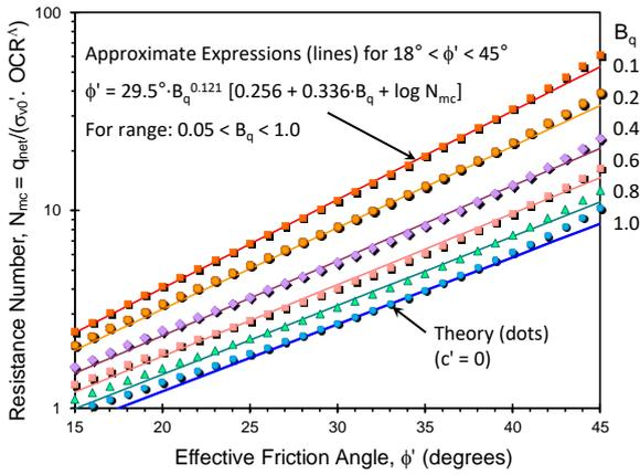
Figure 8 Approximate modified NTH method for evaluating  $\phi'$  in intact clays
