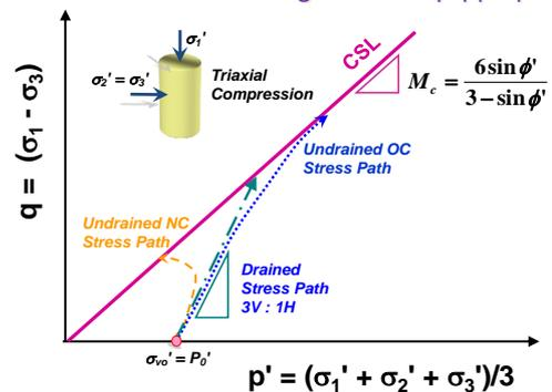
Figure 1 Schematic plot showing stress path from triaxial compression test
