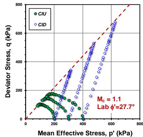
Figure 2 Triaxial compression tests on Korean soft clay- drained and undrained series (data from Lee et al. 2000)
