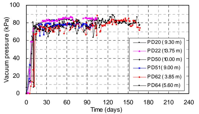
Figure 34 Measured vacuum pressure in PVDs during mass construction using VCM-MT technique
