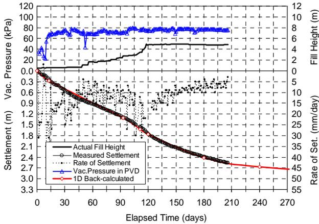
Figure 36 Settlement versus time of Section D1
