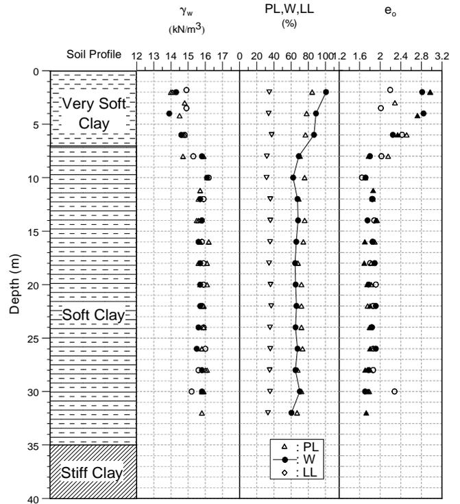
Figure 19a Basic properties of soft clay at CMIT site
