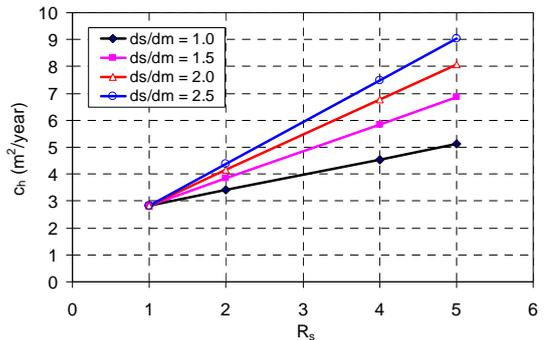
Figure 45 Back-calculated  $c_h$  values for PM3-CM
