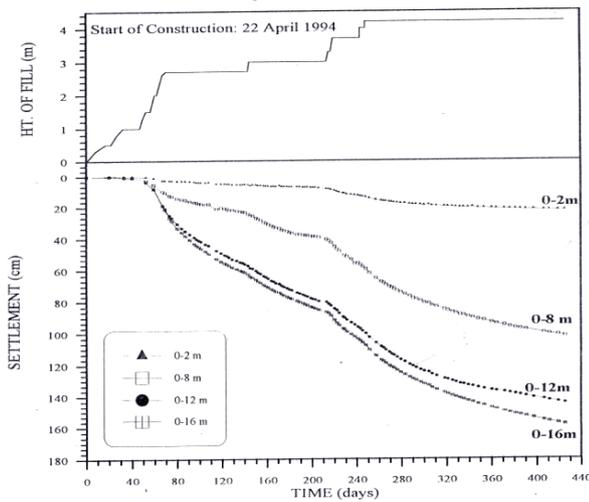
Figure 48 Measured settlements in TS3 – SBIA
