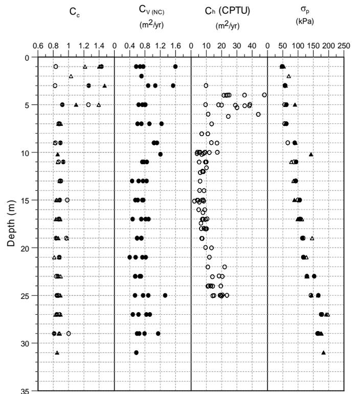
Figure 19b Deformation parameters at CMIT site
