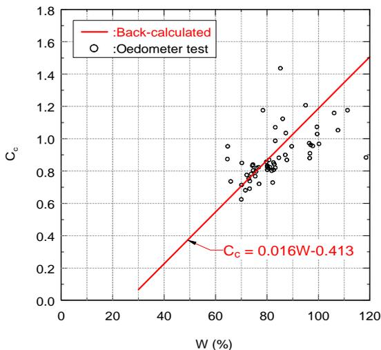
Figure 38 Relation of  $C_c$  versus  $\omega$  for NSEW site
