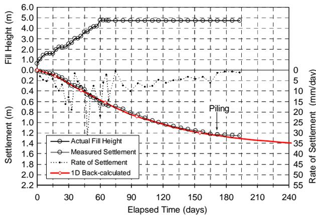
Figure 42 Settlements versus time for PM3-CM
