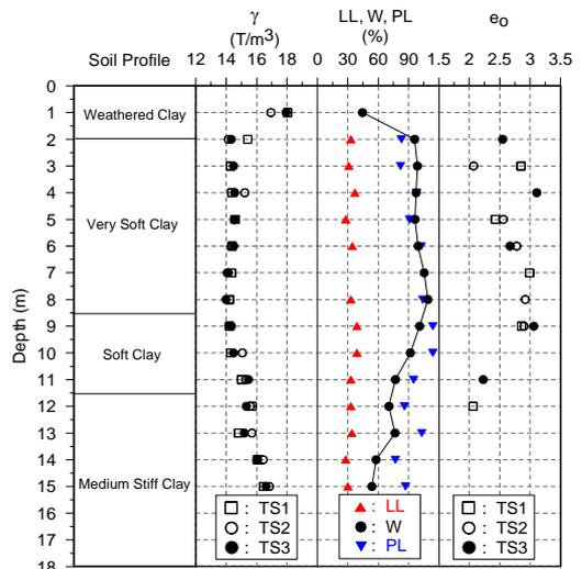
Figure 46 Basic properties of soft soils at SBIA
