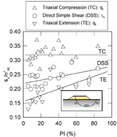
Figure 15 Undrained strength anisotropy from  $CK_0U$  tests on NC clays and silts (Ladd, 1991)
