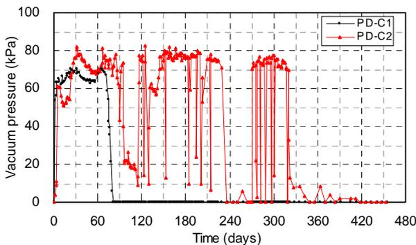
Figure 32 Measured vacuum pressure in PVD (C1 and C2 Sections using VCM-DT method)
