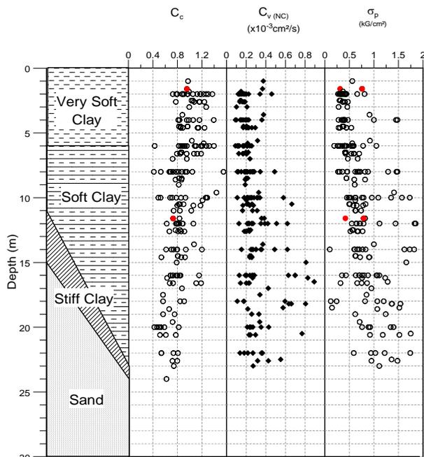
Figure 31 Compressibility properties of GU6-NSEW including D1 Section
