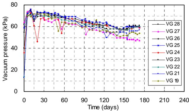
Figure 20 Measured vacuum pressure in sand blanket (CMIT project using VCM-MS method)
