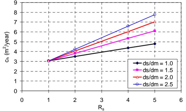
Figure 28 Back-calculated  $c_h$  for Section I - CMIT
