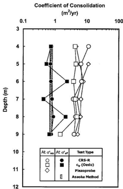
Figure 14 Coefficients of consolidation for soft clay at SBIA site using  $d_s/d_w = 2$  and  $k_h/k_s = 1.4$  for back calculation of  $c_h$  (Seah et al., 2004)
