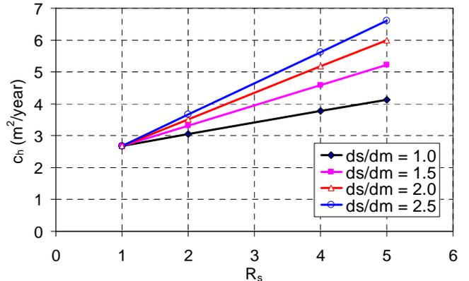
Figure 29 Back-calculated  $c_h$  values for Section II
