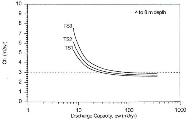
Figure 13 Back-calculated  $c_h$  value of TS1, TS2, TS3 embankments at SBIA site using  $d_s/d_m = 2$  and  $k_h/k_s = 5$  (Bergado et al., 2002)
