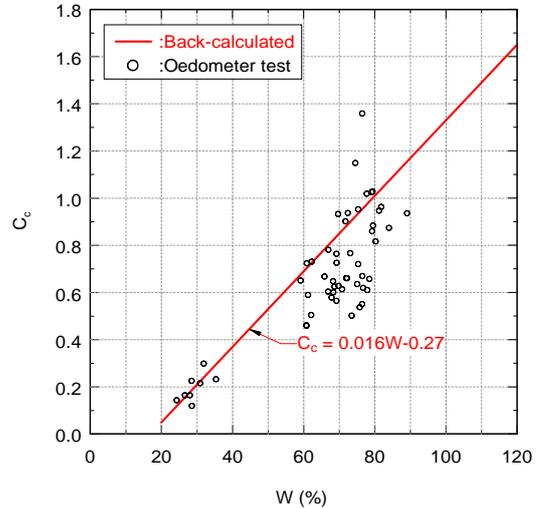
Figure 44 Relation between  $C_c$  versus  $\omega$  for PM3-CM
