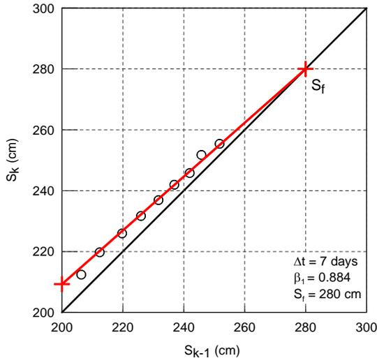
Figure 37 Asaoka plot for Section D1
