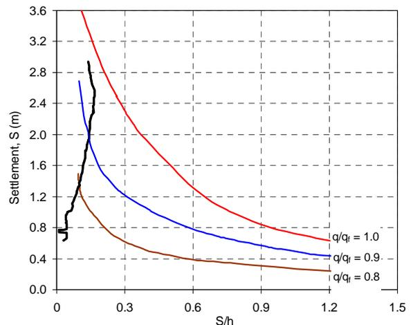
Figure 24 Stability control chart for Section II
