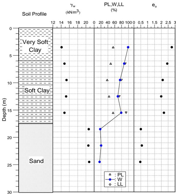
Figure 30 Basic properties at D1 Section – NSEW
