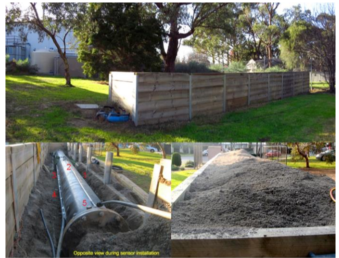
Figure 7 Elevated test area. Large diameter water pipe inside the test area from South end (bottom left) and buried with 0.8m crushed rock (bottom right)
