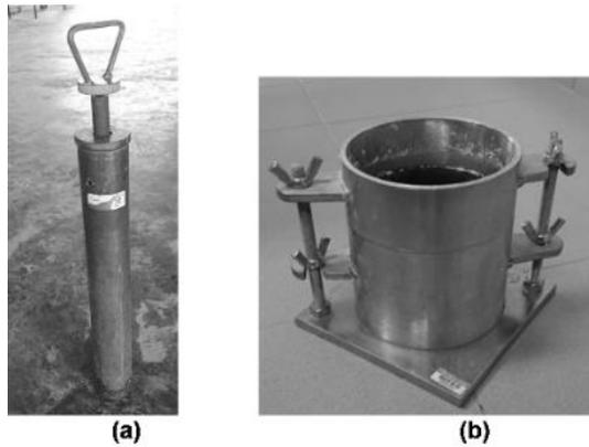
Figure 3 Tools of compaction (a) Standard hammer (b) 6'' mold
